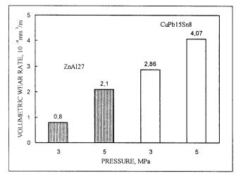
Figure 4. Volumetric wear intensity of the pin in the period of steady state
