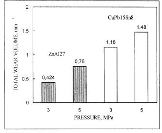
Figure 5. Total wear of pins
