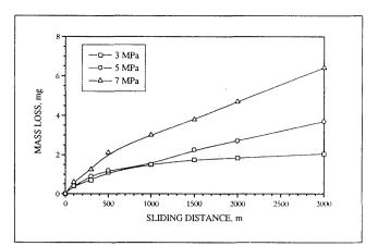
Figure 1. Mass losses of ZnAl 27 vs sliding distance at different loads
