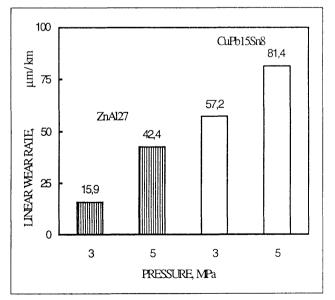
Figure 3. Linear wear intensity of pins in the period of steady state
