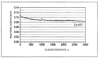
Figure 2. Coefficient of friction vs sliding distance
