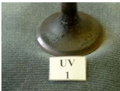
Figure 6: Appearance of the intake valves before and after second modified CEC tests
