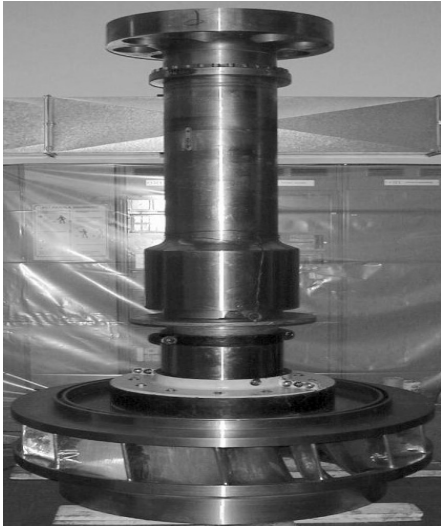
Picture 1. The turbine rotor on the shaft
