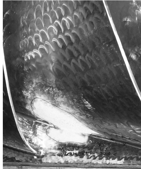
Picture 4. Cavitational damage on the back of the blade No. 2
