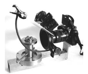
Fig. 3: The custom-made device for circumferential photographing of the discs
