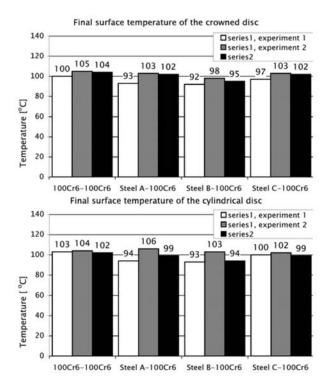
Fig. 13: Final surface temperature near the contact area
