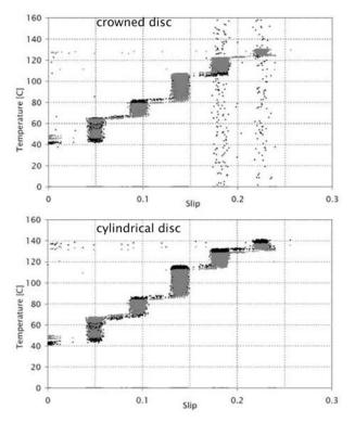
Fig. 7: Temperature measured from a trailing thermocouple (grey) and an embedded thermocouple located 2mm beneath the surface (black). The differences are less than the measurement accuracy
