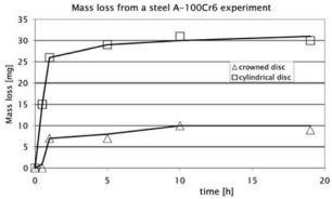
Fig. 9: Typical mass loss over time chart. The running in period (first hour) is clearly seen
