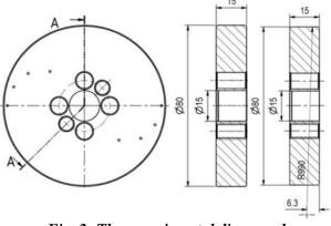
Fig. 2: The experimental discs used
