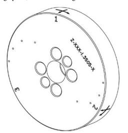
Fig. 4: Illustration of a test discs with the three predefined points of roughness measurements marked. The two different directions (along and across sliding speed) are marked with arrows
