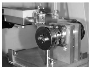
Fig. 5: The roughness measurements custommade device. In front is shown the reference disc, while in the background is shown the measured disc and the measuring stylus
