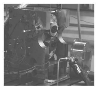
Fig. 1: The two-disk test rig with parallel shafts of the Laboratory of Machine Elements and Machine Design
