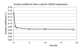
Fig. 11: Typical friction coefficient over time chart. The friction coefficient is rapidly decreased during running-in and then is practically stabilized
