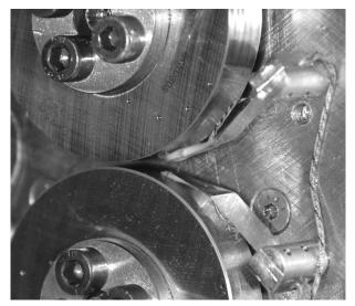
Fig. 6: Trailing thermocouples on the test discs surface. It should be noticed that the thermocouples are located as close as possible to the contact area
