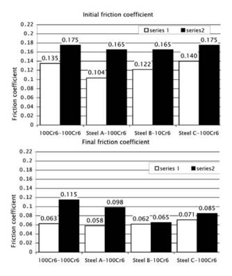
Fig. 10: Initial and final friction coefficient
