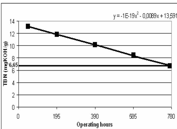
Fig. 8: Extrapolation analysis result and limit value of Total Base Number (TBN)
