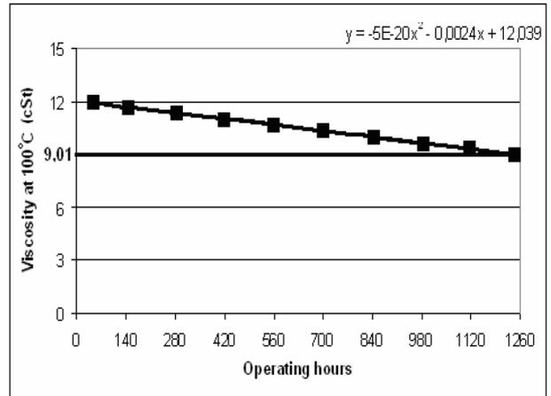
Fig. 10: Extrapolation analysis result and limit value of Viscosity (100°C)
