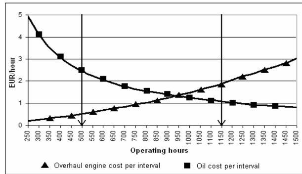
Fig.3: Overhaul engine and oil costs per interval and operating hours profile in engine
