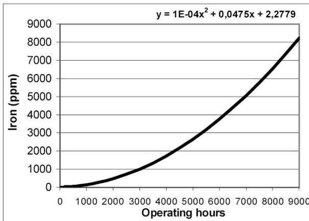
Fig 2: Iron wear debris concentration extrapolation analysis.
