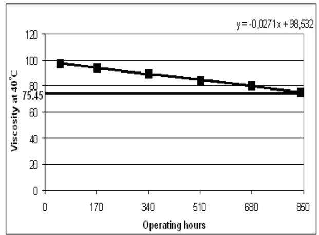
Fig. 9: Extrapolation analysis result and limit value of Viscosity (40°C)
