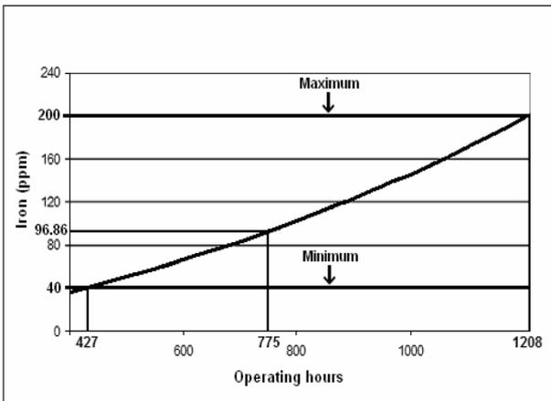
Fig. 7: Extrapolation analysis result and limit values of Iron (Fe)
