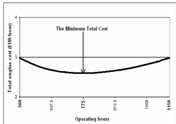
Fig.5: Total engine cost per interval for an optimum oil change point in engine.
