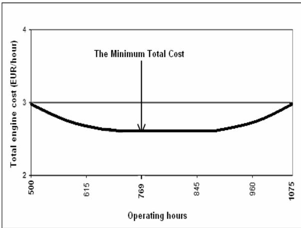
Fig. 6: Total engine cost per interval for an optimum oil change point in the second main Diesel engine.
