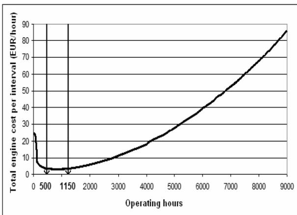
Fig.4: Total engine cost per interval and operating hours profile
