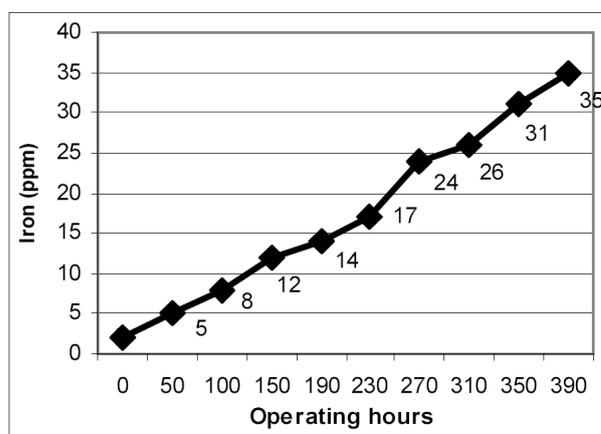
Fig 1: Iron wear debris concentration and operating hours profile.
