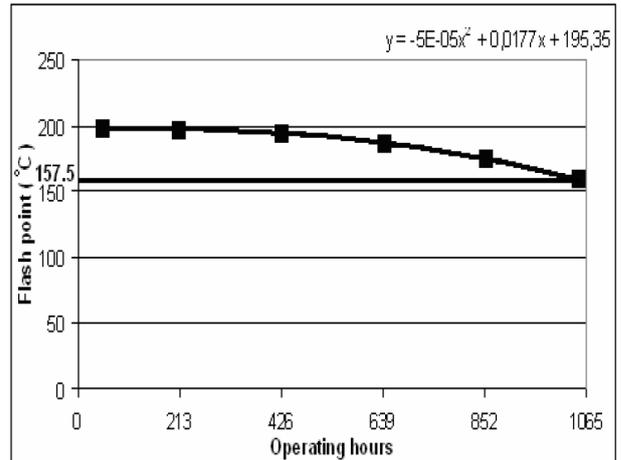
Fig. 11: Extrapolation analysis result and limit value of Flash Point
