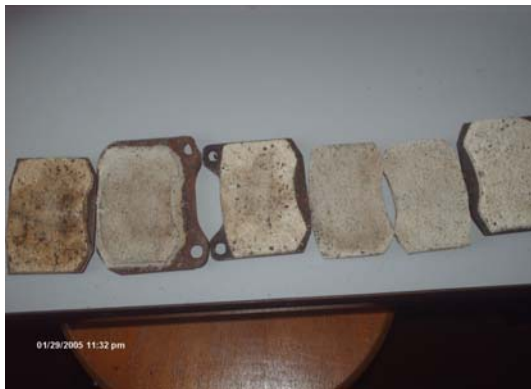
Figure 16. Produced bagasse brake pads
