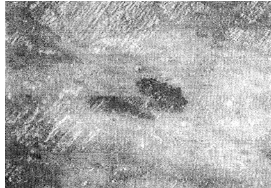
Figure 4. Microstructure of 100 \mu m sieve grade sample(X100). Showing Uniform dark region of resin and white region of bagasse.
