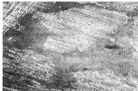
Figure 5. Microstructure of 150 \mu m sieve sample(X100). Showing slight uniform dark region of resin and white region of bagasse.
