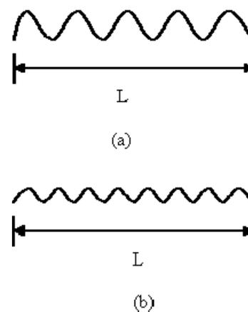
**Figure 7.** (a) The points of contact of a body with low natural frequency, (b) The points of contact of a body with high natural frequency for constant length of contact (L)
