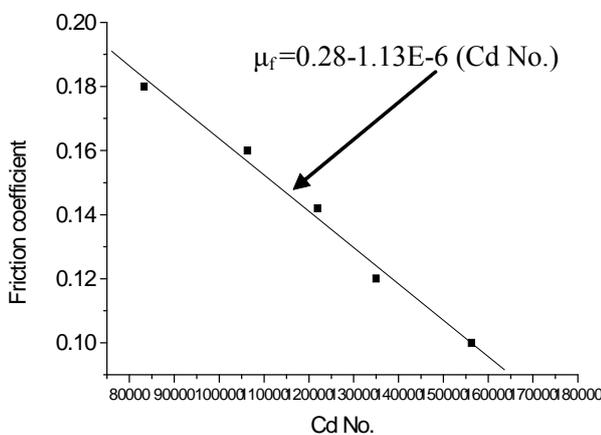
**Figure 8.** Friction coefficient as a function of chowdhury no.
