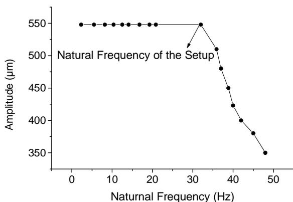
**Figure 3.** Amplitude vs. frequency curve of the setup for 50 kg added dead load
