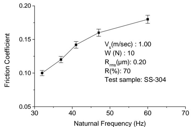
**Figure 6.** Variation of friction coefficient with the variation of natural frequency of the experimental setup for SS-304
