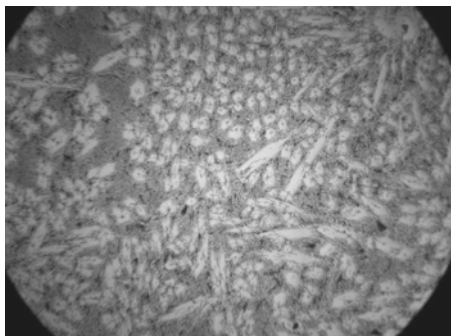
b) Carbides in martensitic base (500×)
