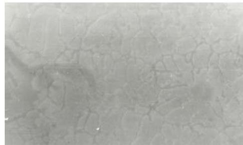
**Figure 2.** Microstructure of the unreinforced Al-4.5Cu Alloy (grey) magnification x 125
