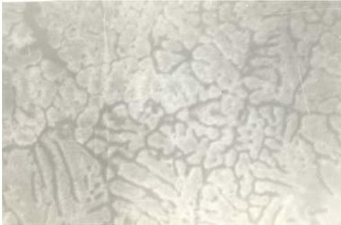
**Figure 6.** Microstructure of Al-4.5Cu alloy reinforced 20% ZrSiO<sub>4</sub>. ZrSiO<sub>4</sub> particles (black) magnification x 125
