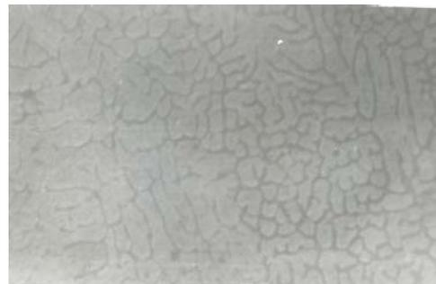
**Figure 3.** Microstructure of the reinforced Al-4.5Cu alloy (5% ZrSiO<sub>4</sub>). Finer grains and thicker grain boundary with little Patches of ZrSiO<sub>4</sub> magnification x 125
