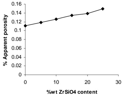
**Figure 8.** Variation of percentage of apparent porosity with weight percentage of ZrSiO<sub>4</sub> content
