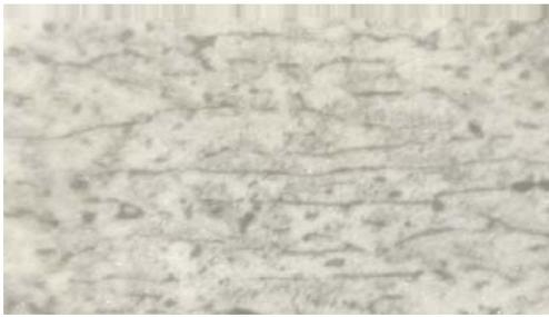
**Figure 5.** Microstructure of Al-4.5Cu alloy reinforced with 15% ZrSiO<sub>4</sub>. Uniform distribution of ZrSiO<sub>4</sub> (black) particles. Magnification X 125
