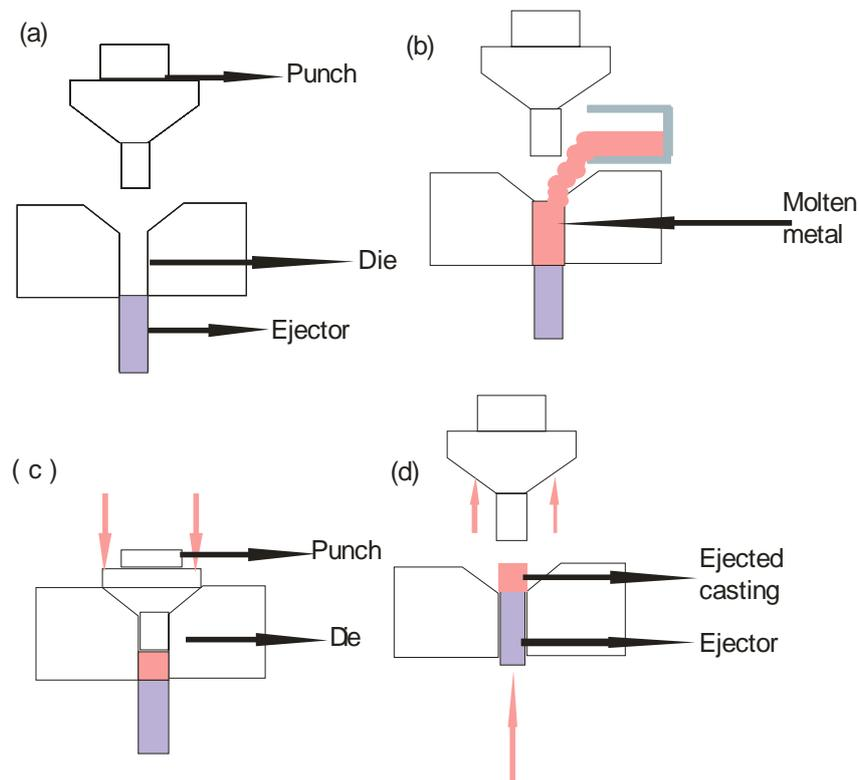
**Figure 1.** Schematic, showing the sequence of steps during squeeze casting operation (a) Pre-heated die and punch. (b) Molten metal poured into the die cavity. (c) Application of squeeze pressure. (d) Ejection of solidified casting
