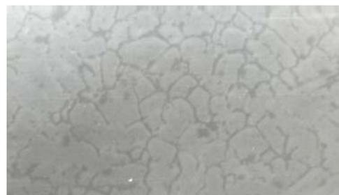
**Figure 4.** Microstructure of Al-4.5Cu alloy reinforced with 10% ZrSiO<sub>4</sub>. More enlargements of the grain boundaries with larger patches of ZrSiO<sub>4</sub> (black) magnification x 125
