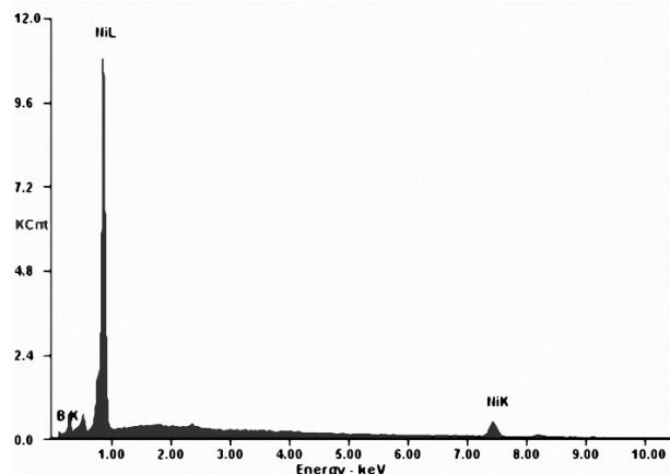
**Figure 6.** EDX spectra of Ni-B coating
