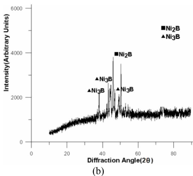
**Figure 8.** XRD patterns of electroless Ni–B deposit
