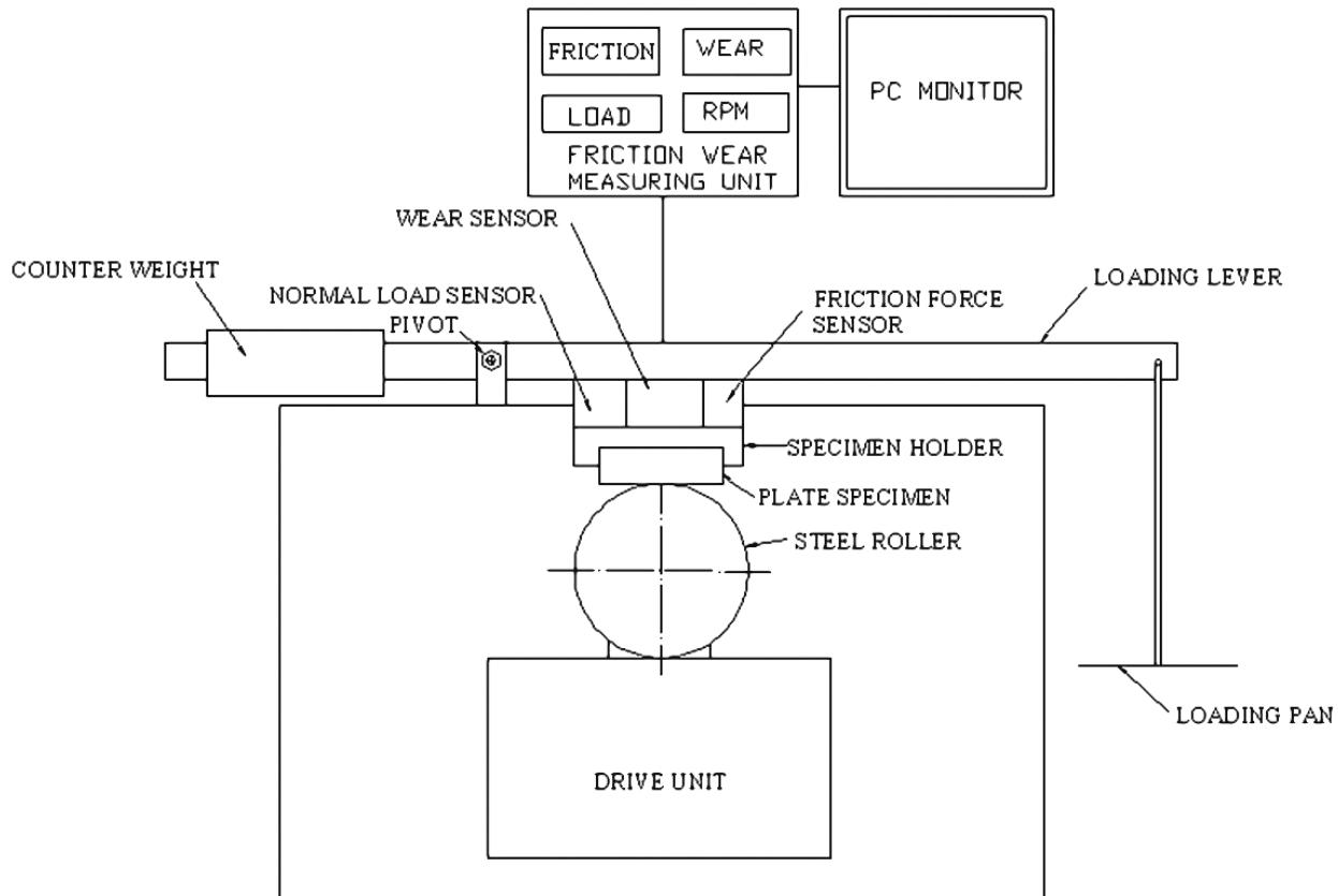
**Figure 3.** Schematic diagram of the multi-tribotester
