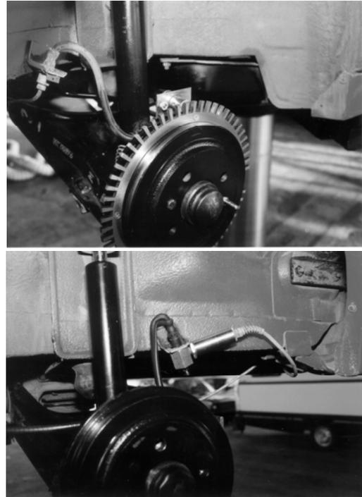
**Figure 12.** Measuring wheel speed and pressure in the rear brake cylinder
