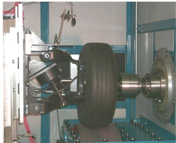
Figure 8. Brake inertial dynamometer
