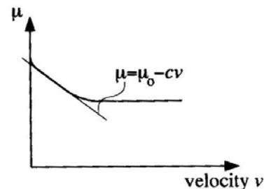
**Figure 3.** Friction characteristics when "negative damping" is possible
