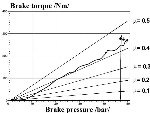
**Figure 15.** Comparative analysis of measured and analytically determined brake torque aimed at determination of friction coefficient fully loaded vehicle at  $v_0 \approx 40$  [km/h]
