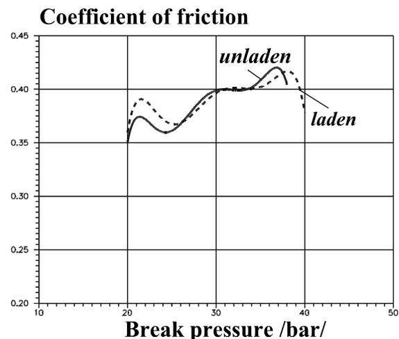
**Figure 13.** Variation of friction coefficient with the variation of pressure for unloaded and fully loaded vehicle at initial speed of  $80 [km/h]$
