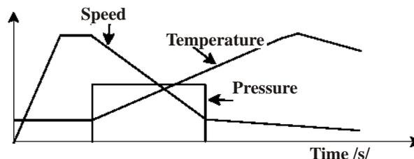
**Figure 10.** Variations of characteristic values during cold brake tests
