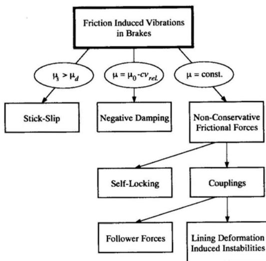
**Figure 1.** Categorization tree for friction induced vibrations in brakes
