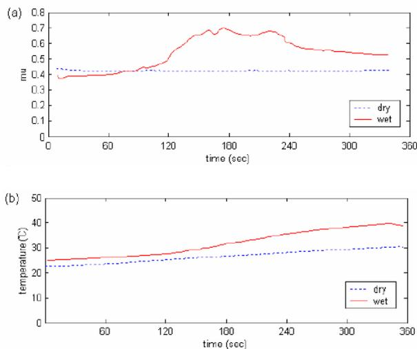
**Figure 9.** Results of the lining friction test at wet and dry conditions: (a) coefficient of friction, (b) temperature
