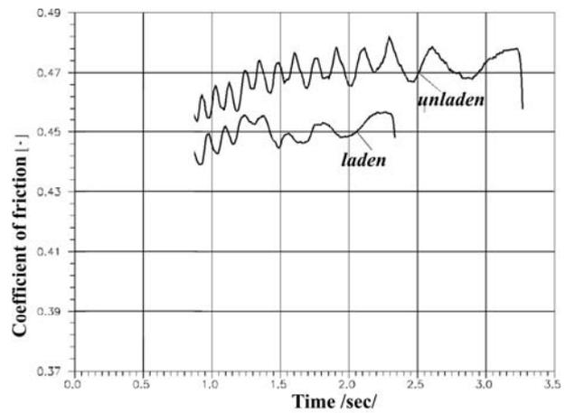
**Figure 16.** Variation of friction coefficient during brake test at  $v_0 \approx 40$  [km/h]
