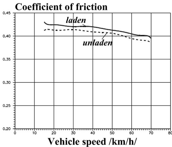
**Figure 14.** Variation of friction coefficient with variation of speed for unloaded and fully loaded vehicle for speeds up to 80 [km/h]
