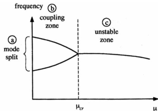
**Figure 6.** Coupling of modes in actuated brake as function of coefficient of friction
