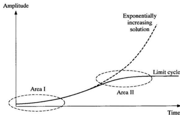
**Figure 5.** Schematic envelope of growing unstable vibration
