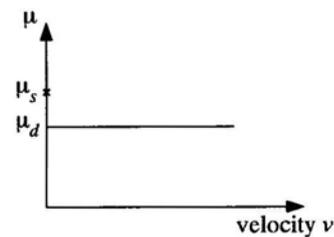
**Figure 2.** Friction characteristic when stick-slip is possible
