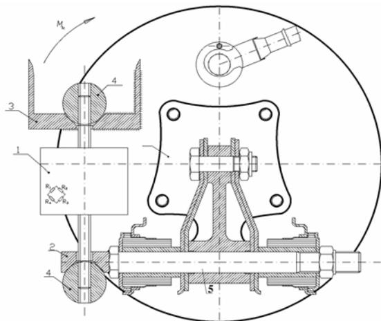
**Figure 11.** Design solutions of brake torque transducers indirectly, through force transducer
