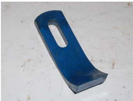
**Figure 2.** A new blade for vegetation and grass cutting
