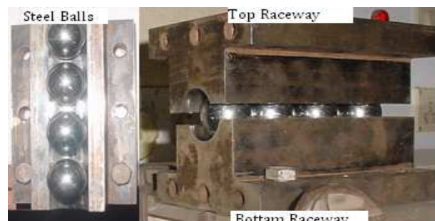
Fig. 1. Linear Model Mock-up bearing assembly.
