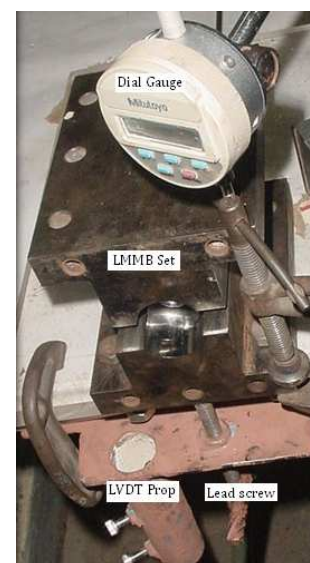
Fig. 3. Experimental set-up for Gravitation-based Method.
