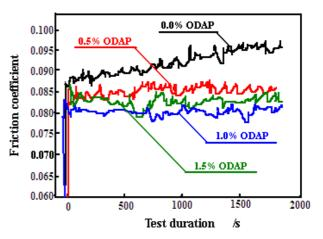
Fig.6. Friction coefficients versus test durations
