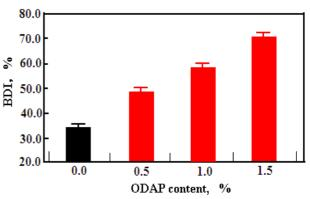
**Fig. 2.** Biodegradability of HVI 350 lubricating oil against contents of ODAP.
