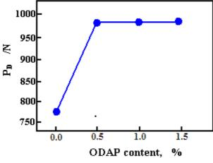
Fig. 4. Welding loads versus ODAP contents.
