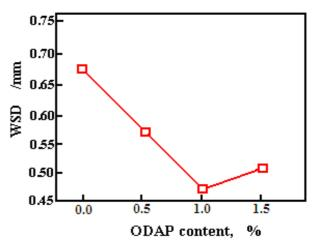
Fig. 5. Wear scar diameters versus ODAP contents.
