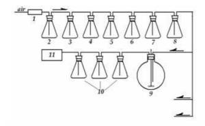
1—air flowmeter; 2—buffer ; 3,4,5,6—CO<sub>2</sub> degasser; 7—CO<sub>2</sub> examiner; 8—buffer; 9—bioreactor; 10—CO<sub>2</sub> absorber; 11—titrator
