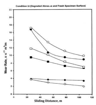
**Fig. 5.** Wear rate of the specimens as a function of sliding distance at various applied loads in experimental condition (open symbols: composite; closed symbols: matrix alloy,  $\blacklozenge: 1 \text{ N}, \blacksquare: 3 \text{ N}, \blacktriangle: 5 \text{ N}, \circlearrowright: 7 \text{ N} [13].$
