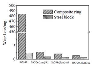
**Fig. 12.** Wear loss of the composites and counterfaces of wear process for SiC/Al and SiC/Gr/Al [27-29].
