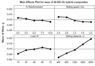
**Fig. 10.** Main effect plot of effect of factors on wear of Al-SiC-Gr hybrid composites [23-25].
