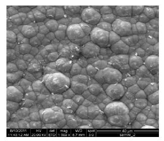
Fig. 5. SEM image of Ni-P-W coated surface
