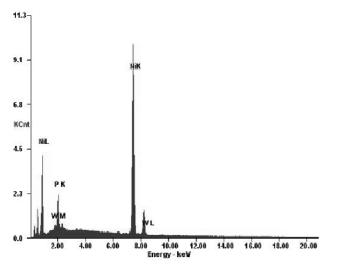
Fig. 4. EDX spectra of coated surface.
