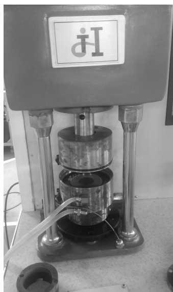
Fig. 10. Shear film strength testing device.
