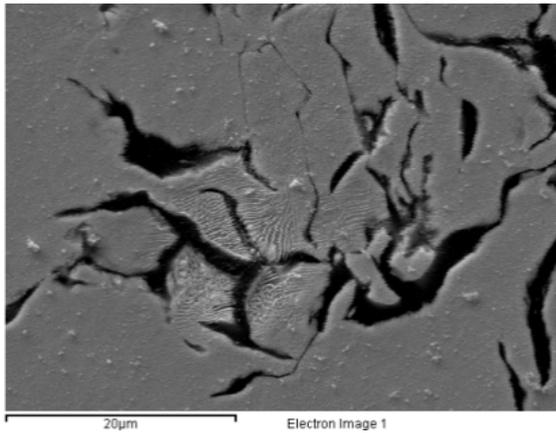
**Plate 1.** SEM Micrographs of grey cast iron with Manganese additions 0.24 % Mn.
