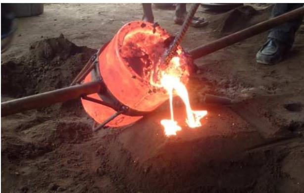
**Plate C.** Pouring into the mould
