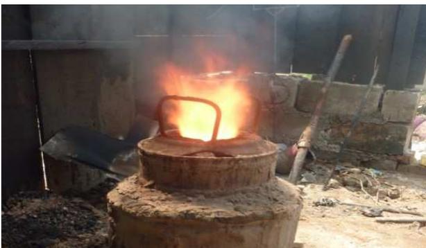
**Plate B.** The 40 kg crucible furnace.
