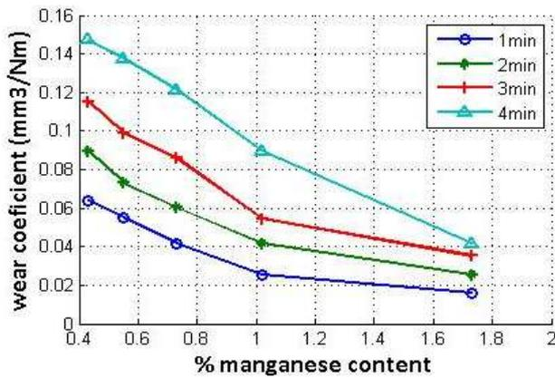
Fig. 1. Change in wear coefficient with increasing time.
