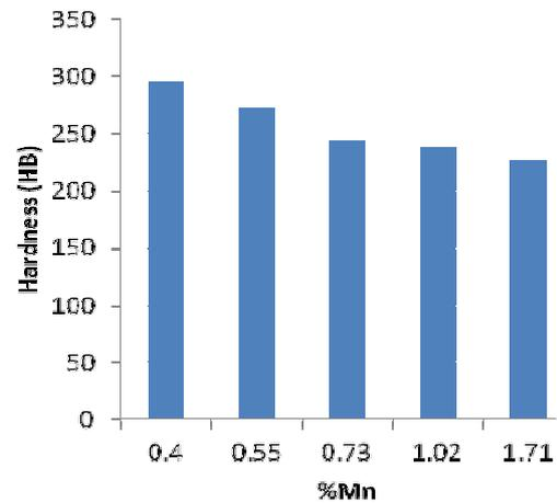
Fig. 5. Hardness of the different compositions of grey cast iron.
