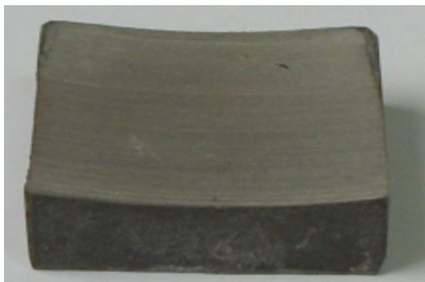
Fig. 2. Wear resistance test sample.
