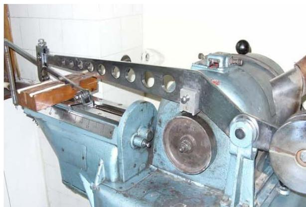
Fig. 3. Tribological and Wear resistance testing device.
