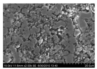
**Fig. 2.** Micro graph of heat treated manganese phosphate coated AISI D2 steel.
