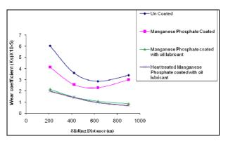
**Fig. 3.** Wear coefficient vs sliding distance at velocity of 3.0 m/s.
