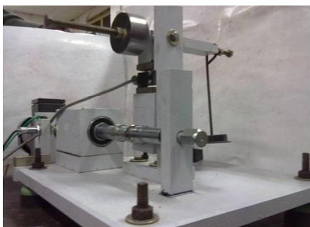
Fig. 1. Schematic diagram of micro abrasion tester.
