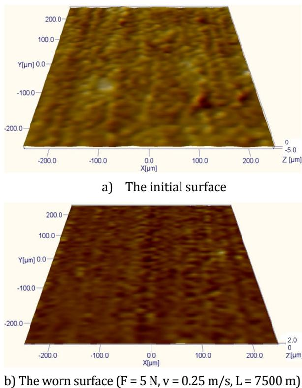
**Fig. 2.** Virtual images of the polymeric blocks made of PBT + 10 % PTFE.
