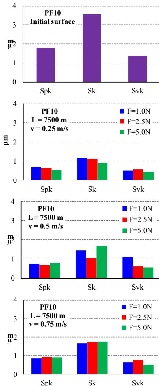
Fig. 4. The influence of the normal force on the average values of the dimensional amplitude parameters for the blocks made of PF10.
