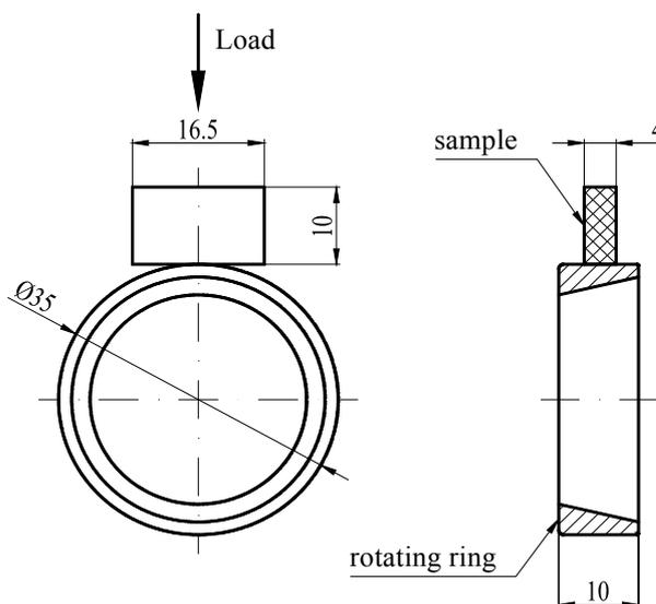
**Fig. 1.** The shapes and dimensions of the friction couple block-on-ring.
