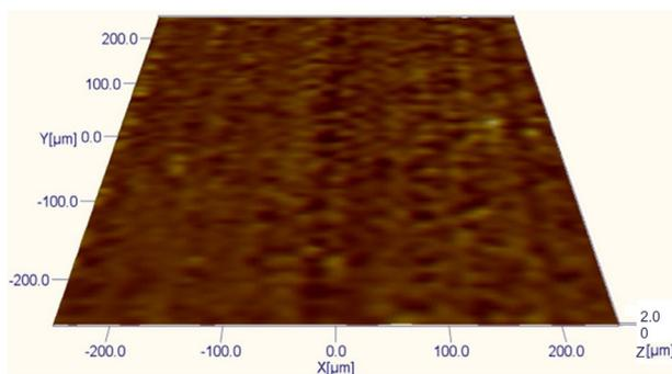
b) The worn surface ( $F = 5 \text{ N}$ ,  $v = 0.25 \text{ m/s}$ ,  $L = 7500 \text{ m}$ )
