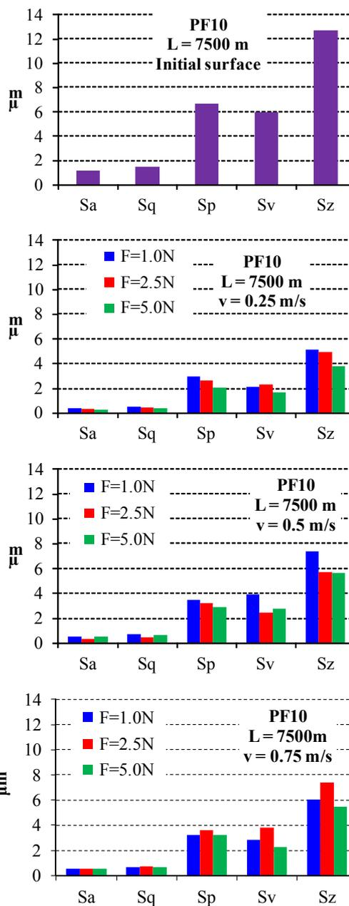
**Fig. 3.** The influence of the normal force on the average values of the dimensional amplitude parameters for the blocks made of PF10 (PBT + 10 % PTFE).
