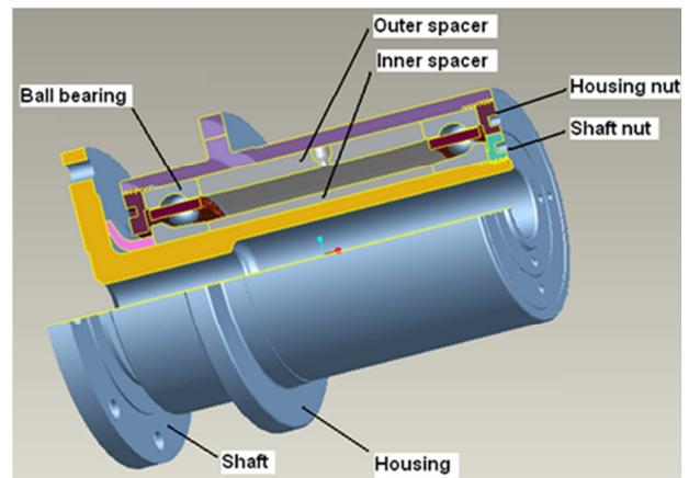
**Fig. 2.** Bearing cartridge assembly.
