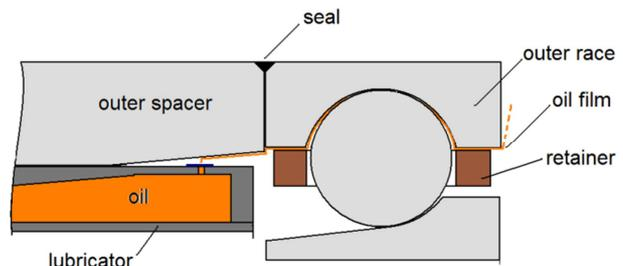
Fig. 6. Schematic view of oil flow from the lubricator.
