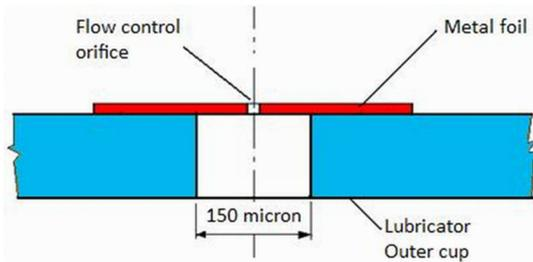
Fig. 7. Arrangement of flow control orifice.
