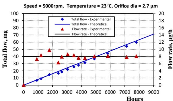
Fig. 9. Theoretical and experimental results of a lubricator with 2.7 µm diameter orifice.
