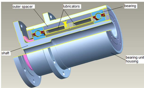
Fig. 5. The bearing cartridge assembly with the lubricators [28].
