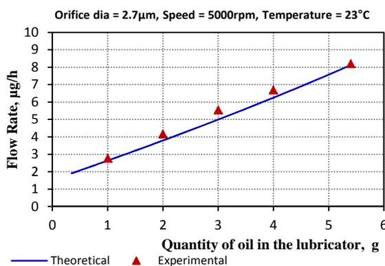
Fig. 11. Variation of theoretical and experimental flow rate with quantity of oil in the reservoir.
