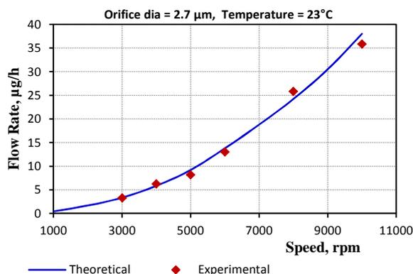
Fig.10. Variation of theoretical and experimental flow rate with operating speed.
