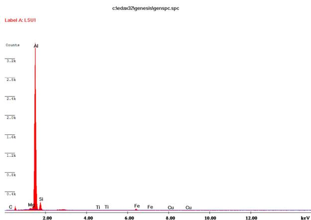
Fig. 5. EDX analysis of worn surface SiC/Gr/Al specimen.
