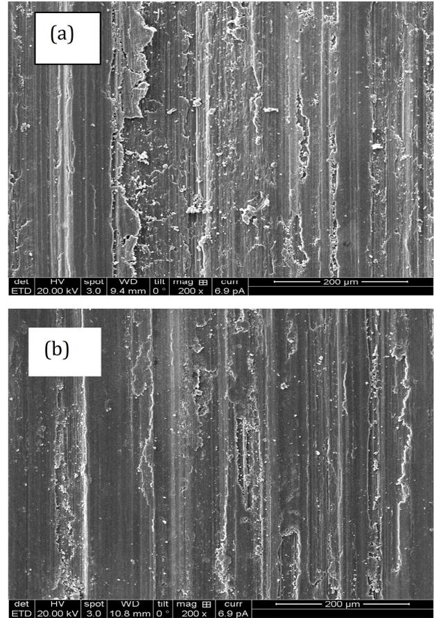
**Fig. 4.** SEM worn surfaces of (a) as-cast (b) heat-treated hybrid composites as a function of constant variables such as load (30 N), sliding speed (3.77 m/s) and sliding distance (4500 m).
