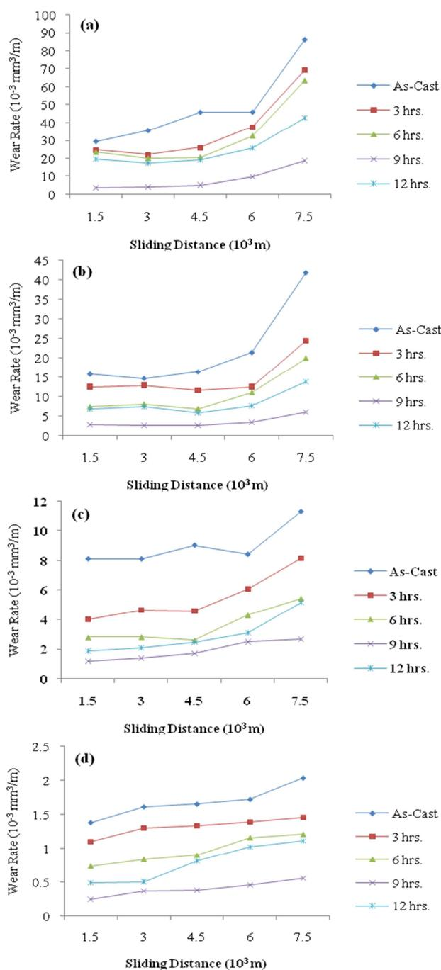
**Fig. 1.** Cumulative wear rate of as-cast and different ageing treated composites as a function of sliding distance at constant sliding speed of 3.77 m/s and applied load of 30 N. (a). A356 alloy (b). A356-3%SiC<sub>p</sub>-3%Gr (c). A356-6%SiC<sub>p</sub>-3%Gr (d). A356-9%SiC<sub>p</sub>-3%Gr.
