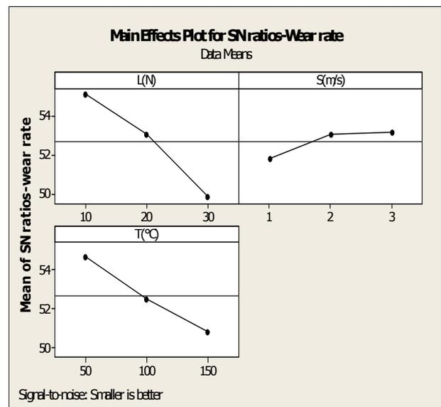
**Fig. 3.** Main Effects Plot for S/N ratio-Wear rate.
