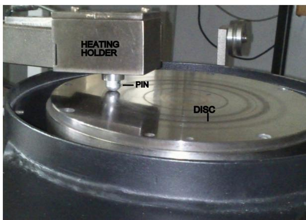
Fig. 1. Pin-on-disc wear tester.
