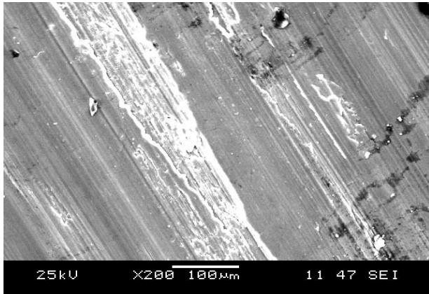
**Fig. 6.** SEM Micrograph for L=20 N, S=1 m/s, T=100 °C.
