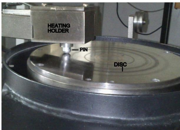
**Fig. 1.** Pin-on-disc wear tester.
