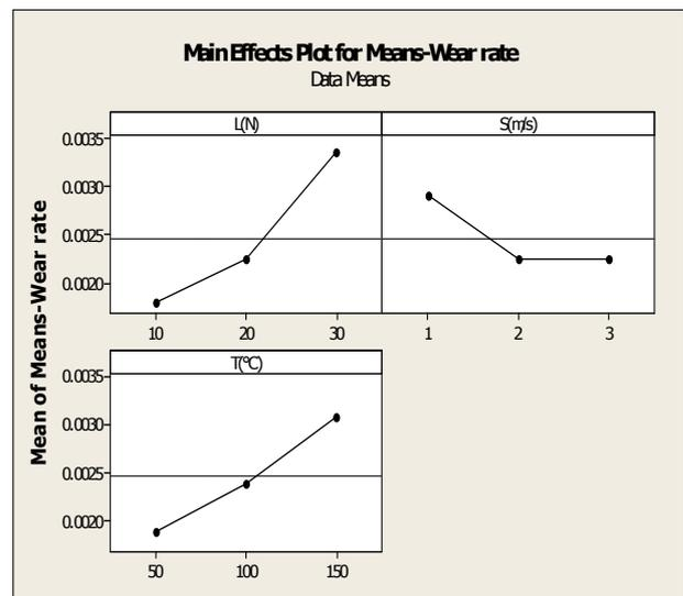
**Fig. 2.** Main effects plot for Means-Wear rate.
