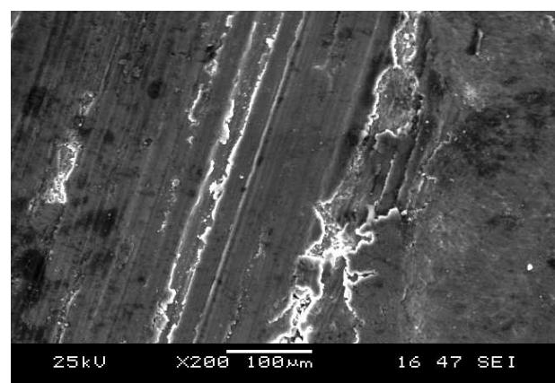
Fig. 4. SEM Micrograph for L=10 N, S=1 m/s, T=50 °C.
