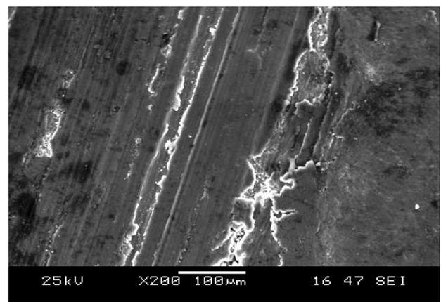
**Fig. 4.** SEM Micrograph for L=10 N, S=1 m/s, T=50 °C.
