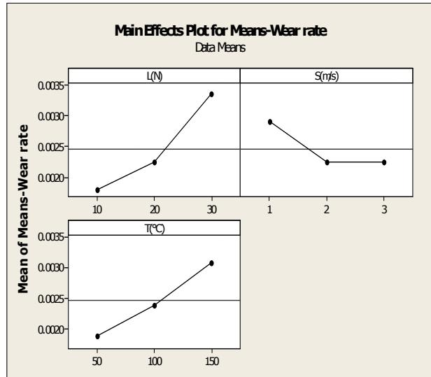
**Fig. 2.** Main effects plot for Means-Wear rate.
