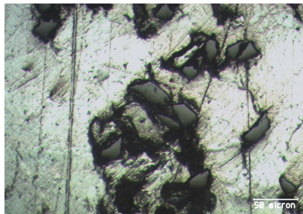
Fig. 2. Microstructure of ZA27/3% SiC/3% Gr composite (magnification x 400).
