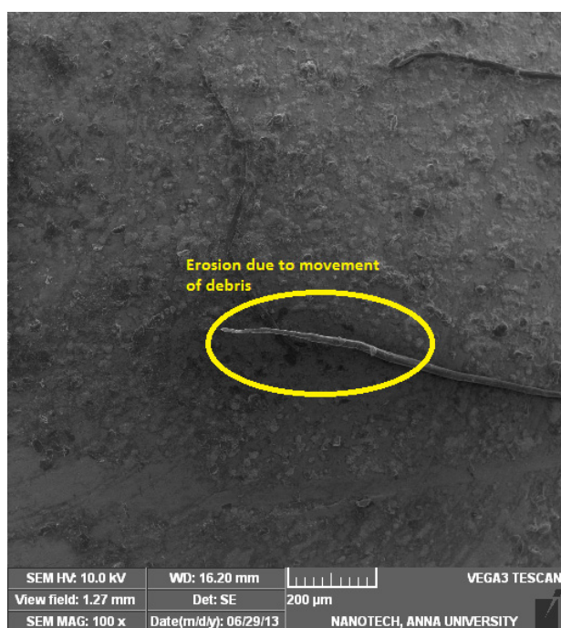
Fig. 7. SEM micrograph of the bearing material lubricated in CMRO with 0.5 % Nano CuO.
