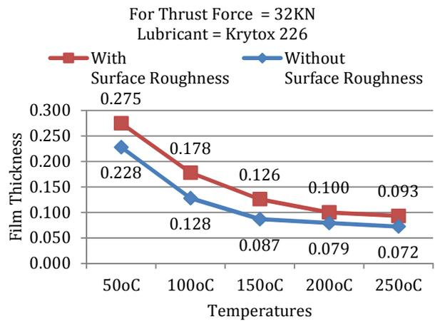
Fig. 8. Effect of surface roughness at 32KN Force for Krytox 226
