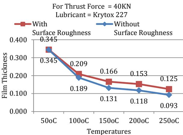
Fig. 7 Effect of surface roughness at 40KN Force for Krytox 227
