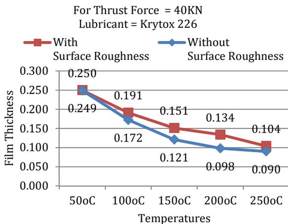
Fig. 6 Effect of surface roughness at 40KN Force for Krytox 226.
