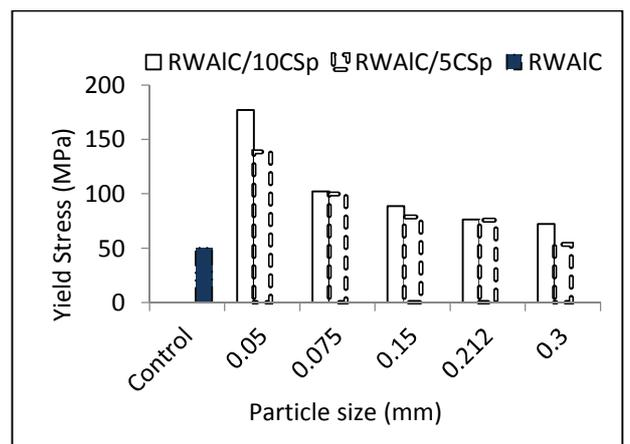
Fig. 6. Yield Stresses of Composites Particulates Size Curve.
