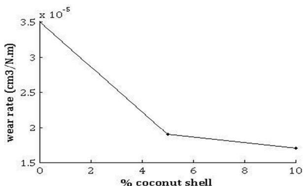
**Fig. 11.** Specific wear rates-% coconut shell at 2.36 ms<sup>-1</sup>.
