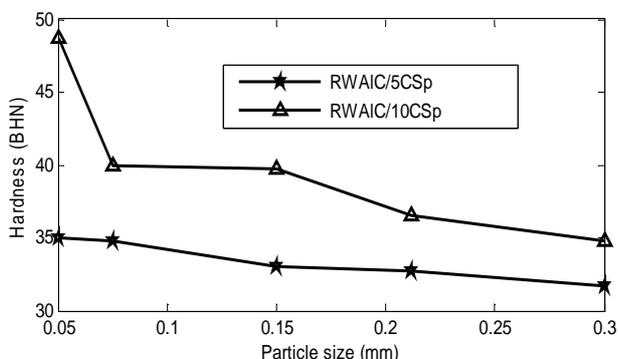
Fig. 7. Hardness Values with Grain Size Curve of the RWAIC/CSp Composites.
