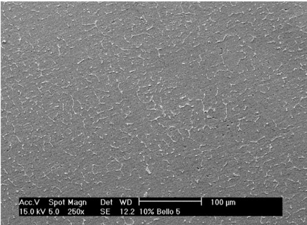
Fig. 3. SEM Micrograph of RWAIC/10CSp (50µm) Composite (X250).
