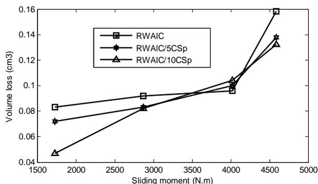
Fig. 10. Volume Loss at 4.72 ms⁻¹ with Sliding Moment Curves.
