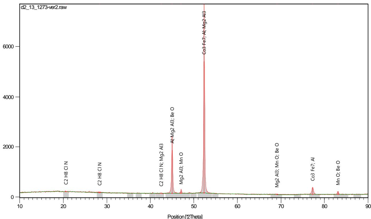
Figure 1. XRD Profile of Elemental Segregation of RWAIC/10CSp Composite.
