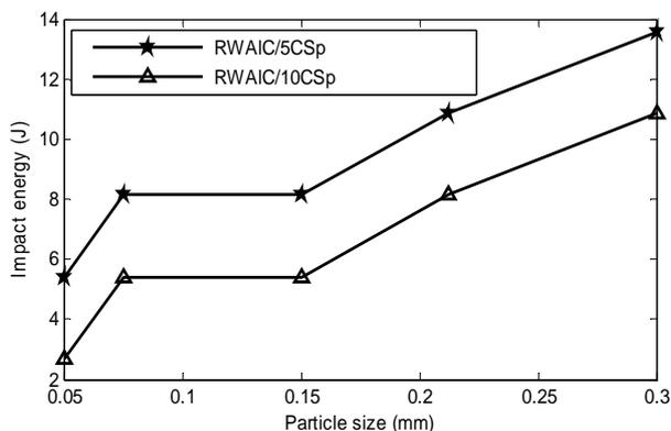
Fig. 8. Impact Energy with Grain Size of RWAIC/CSp.
