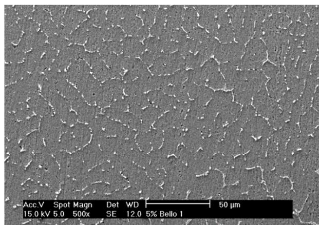
Fig. 2. SEM Micrograph of RWAIC/5CSp (50µm) composite (X500).
