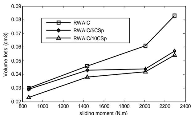
Fig. 9. Volume Loss at 2.36 ms⁻¹ with sliding moment curves.
