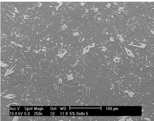
Fig. 4. SEM Micrograph of RWAIC/5CSp (300µm) Composite (X250).
