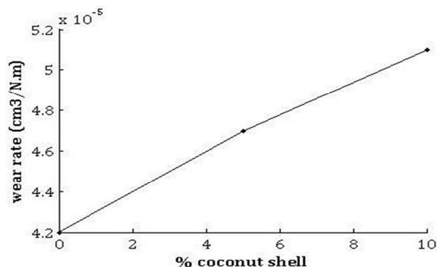
**Fig. 12.** Specific wear rate -% coconut shell at 4.72 ms<sup>-1</sup>.
