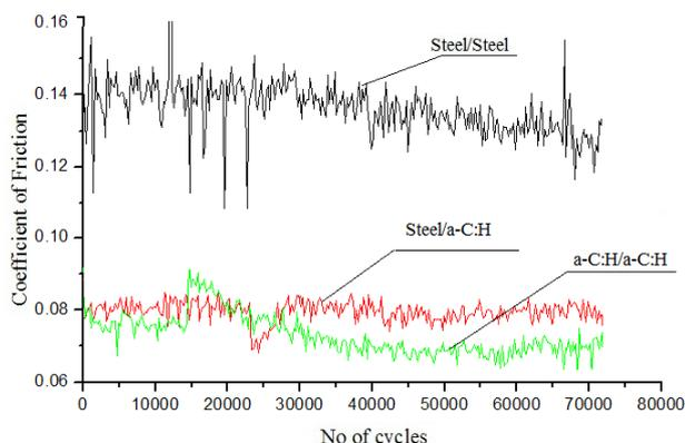
**Fig. 2.** Coefficient of friction of steel/steel, steel/a-C:H and a-C:H/a-C:H combinations with Canola oil lubrication.
