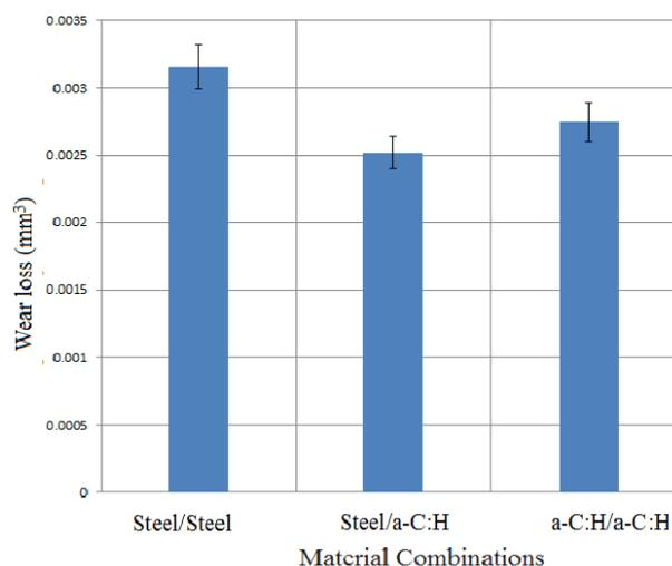
**Fig. 3.** Wear loss of selected ball and disc sets of steel/steel, steel/a-C:H and a-C:H/a-C:H material combinations, when lubricated with Canola oil. Error bars represent  $\pm$  one standard deviation of the measurements.
