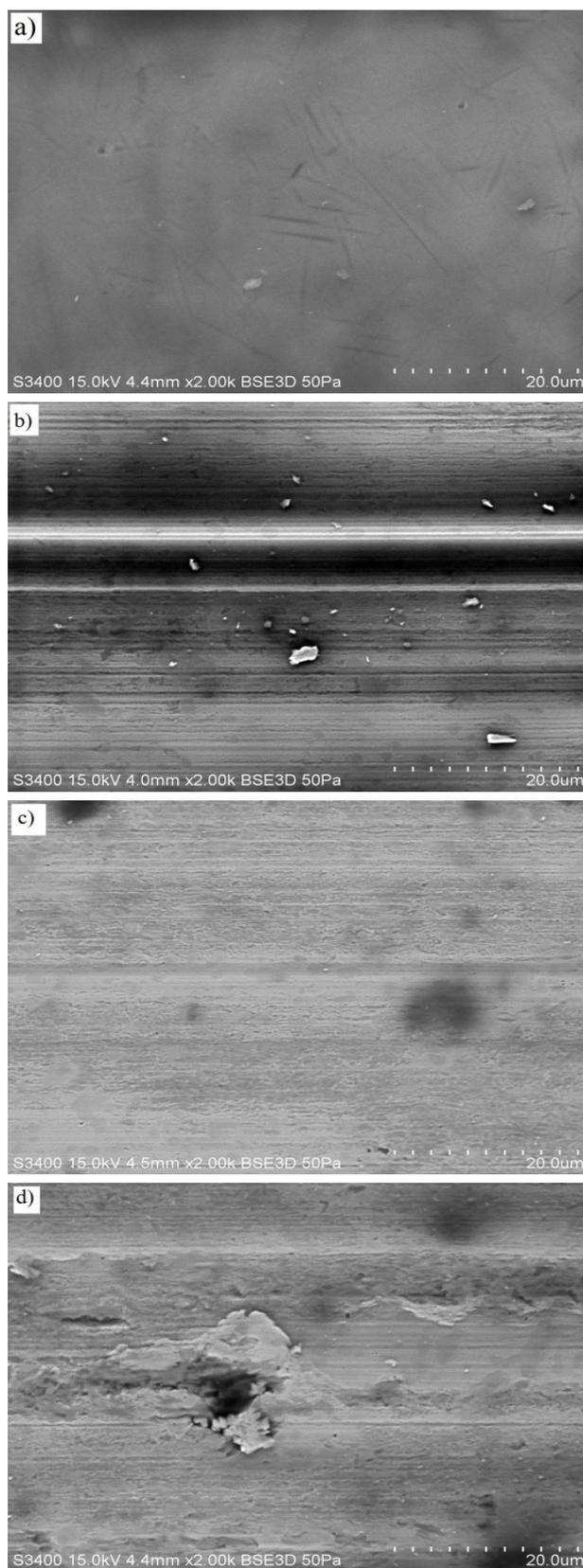
**Fig. 4.** SEM micrographs of the balls surfaces a) deposited surface of a-C:H DLC films; and worn surfaces when lubricated with Canola oil: (b) steel/steel (WSD =  $416 \pm 1.6 \mu\text{m}$ ) (c) steel/a-C:H (WSD =  $318 \pm 1.3 \mu\text{m}$ ) and (d) a-C:H/a-C:H combination (WSD =  $355 \pm 1.1 \mu\text{m}$ ).
