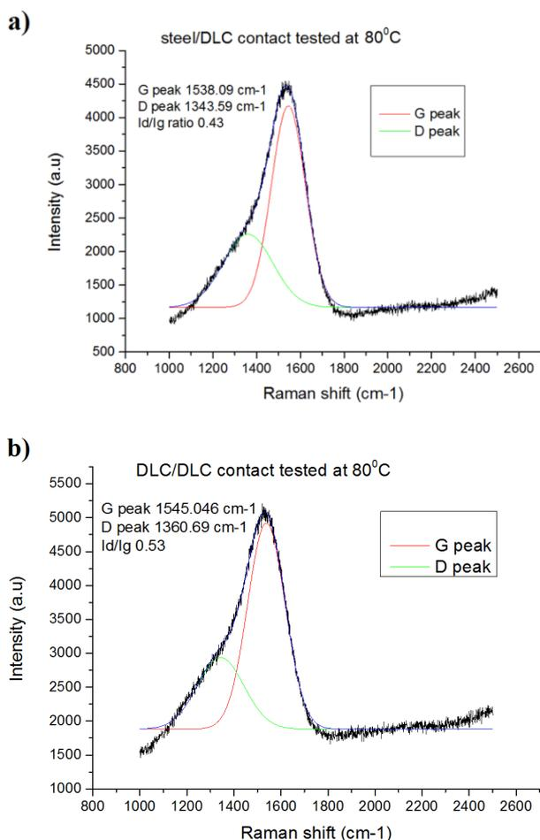
**Fig. 6.** RAMAN analysis of the a-C:H DLC coating wear track.
