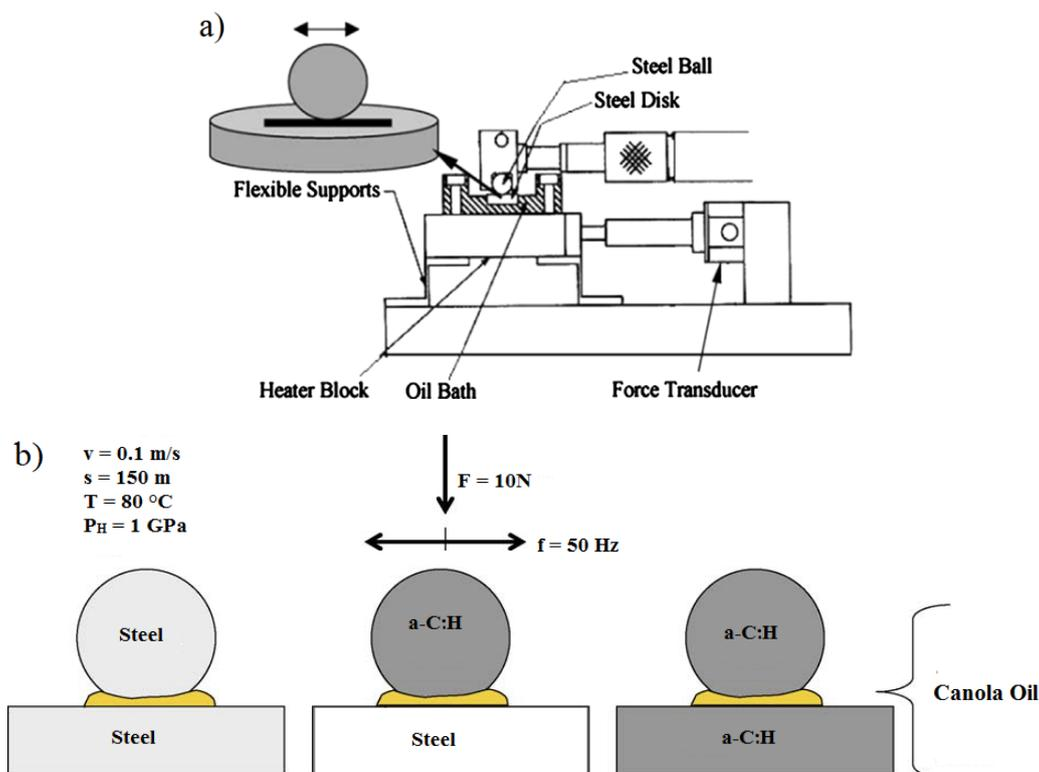
**Fig. 1.** HFRR test: a) schematic diagram of HFRR, b) materials and experimental condition.
