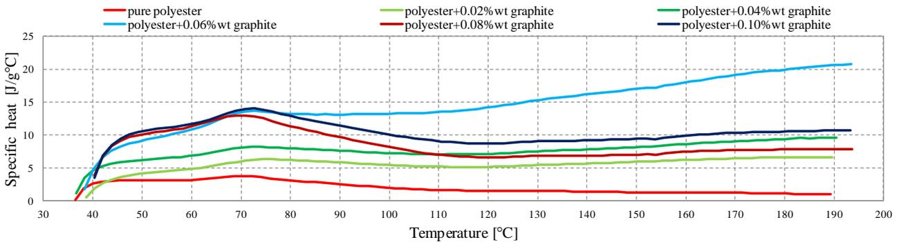
Fig. 6. Specific heat depending on temperature for polyester with graphite composite on heating stage.
