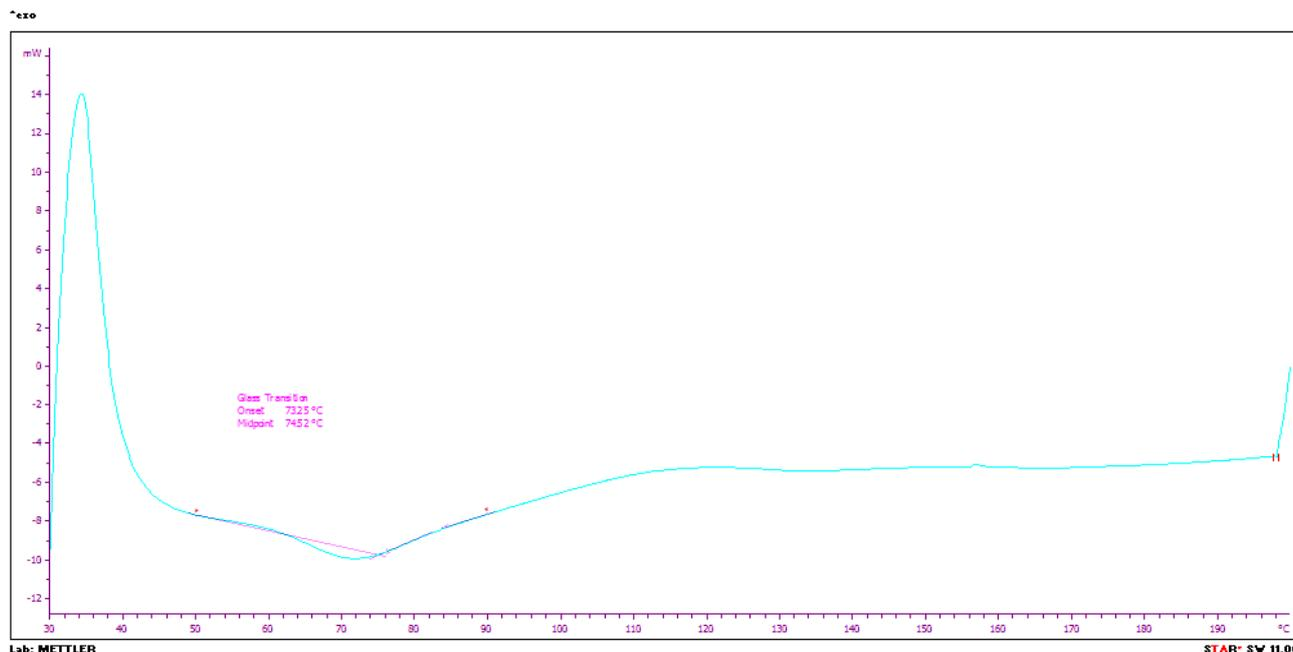
Fig. 12. Determination of glass transition temperature for polyester with 0.04%wt graphene composite.
