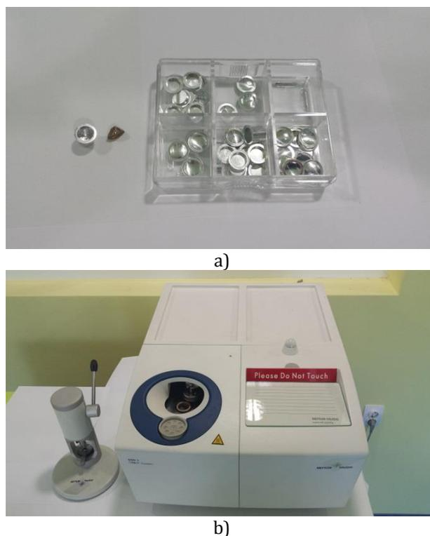
Fig. 1. a) Samples and b) DSC tester.
