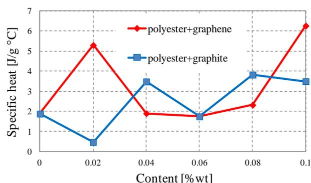
Fig. 9. Specific heat depending on content for polyester with graphene and polyester with graphite composite on heating stage
