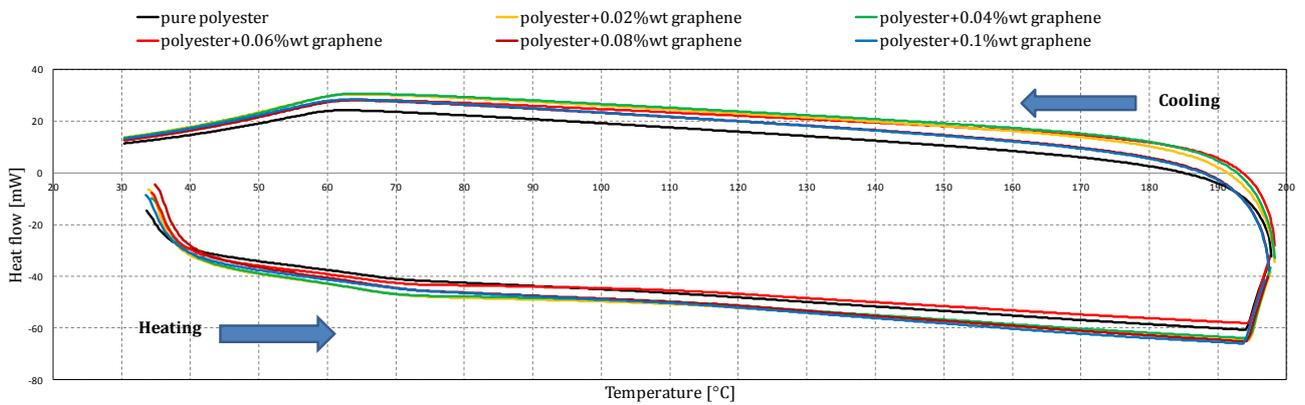
Fig. 5. Heat flow depending on temperature for polyester with graphene composites.
