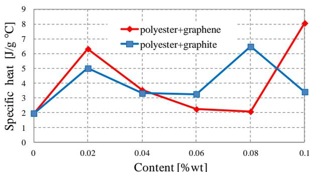
Fig. 10. Specific heat depending on content for polyester with graphene and polyester with graphite composite on cooling stage.
