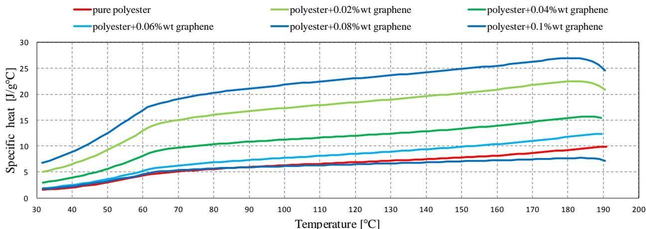
Fig. 3. Specific heat depending on temperature for polyester-graphene composite on cooling stage.
