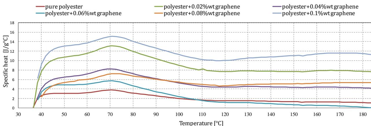
Fig. 2. Specific heat depending on temperature during heating stage for polyester with graphene composite.
