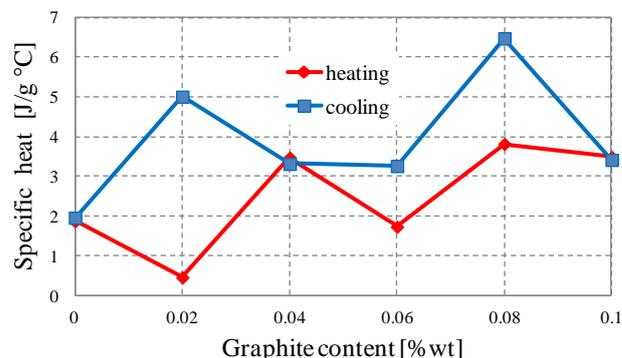
Fig. 8. Specific heat depending on graphite content.
