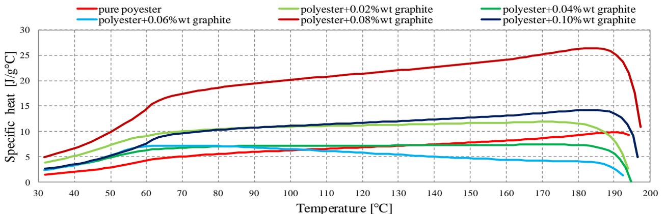
Fig. 7. Specific heat depending on temperature for polyester-graphite composite on cooling stage.
