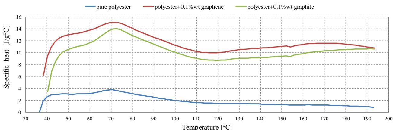
Fig. 11. Specific heat depending on temperature for polyester with 0.1%wt graphene and polyester with 0.1 %wt graphite composite on heating stage.
