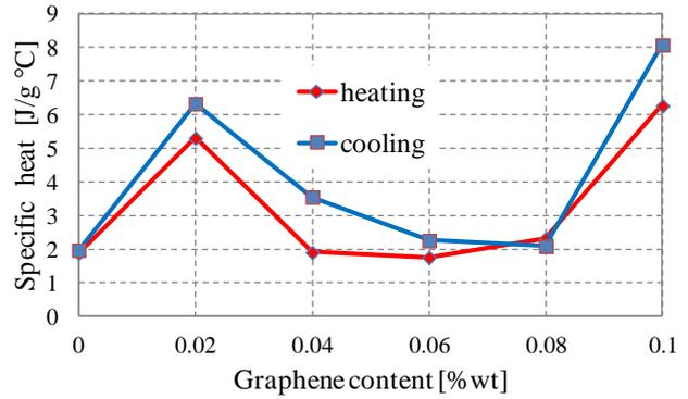
Fig. 4. Specific heat depending on graphene content.
