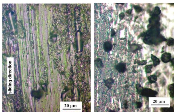
**Fig. 5.** Images by optical microscopy, for  $p=0.5$  MPa and  $v=0.5$  m/s; a) worn surface of disc made from PPS GF40; b) worn surface of steel pin.
