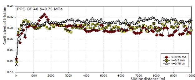
**Fig. 6.** Coefficient of friction in case of PPS GF40 composite, for contact pressure  $p = 0.75$  MPa.
