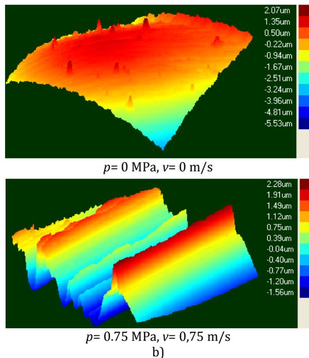
Fig. 12. 3D isochromatic virtual images of initial ( $p=0$  MPa,  $v=0$  m/s), respectively worn surfaces ( $p=0.75$  MPa,  $v=0.75$  m/s); a) PPS GF40 disc; b) steel pin.
