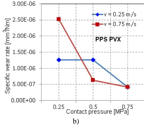
Fig. 9. Specific wear rate depending on contact pressure; a) PPS GF40; b) PPS PVX.
