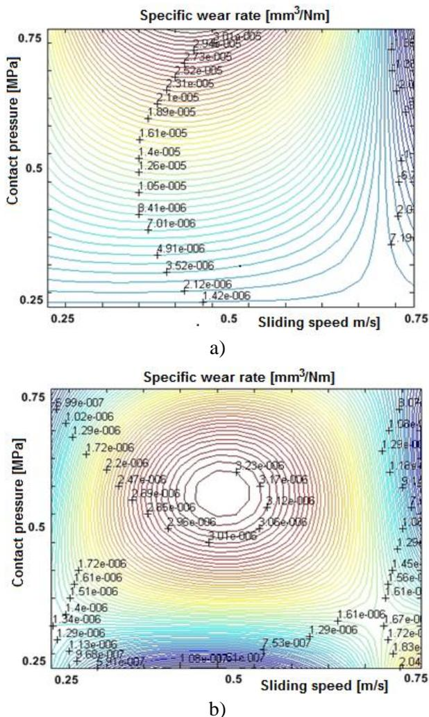
Fig. 11. Contour plots of specific wear rate; a) PPS GF40; b) PPS PVX.
