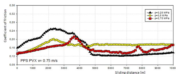
**Fig. 1** Coefficient of friction in case of PPS PVX composite, for test speed  $v = 0.75$  m/s.
