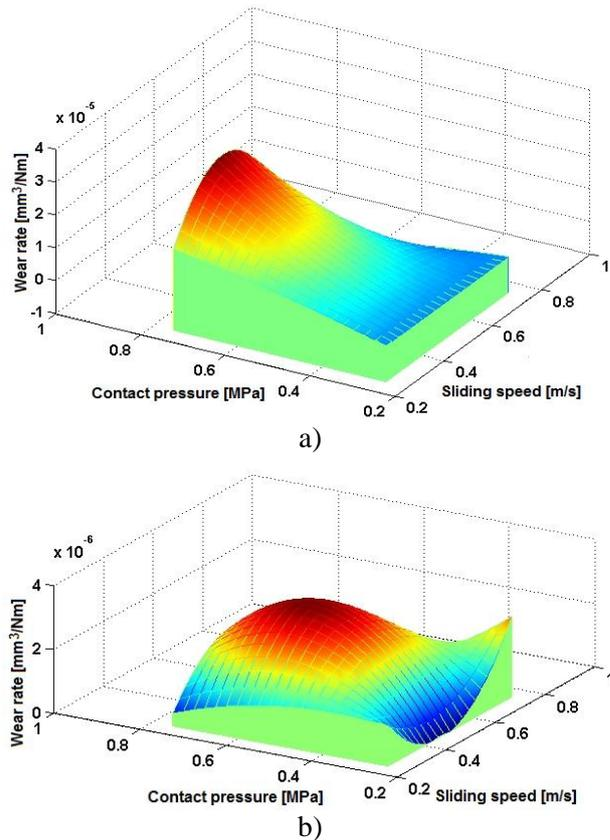
Fig. 10. 3D graphs of specific wear rate after pin-on-disc test; a) PPS GF 40; b) PPS PVX.
