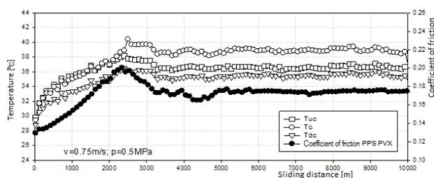
**Fig. 8.** Correlation temperature-coefficient of friction for PPS PVX ( $v = 0.75$  m/s,  $p = 0.75$  MPa).
