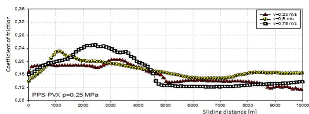
**Fig. 3.** Coefficient of friction in case of PPS PVX composite, for contact pressure  $p = 0.25$  MPa.
