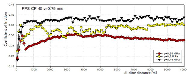
**Fig. 4.** Coefficient of friction in case of PPS GF40 composite, for test speed  $v = 0.75$  m/s.
