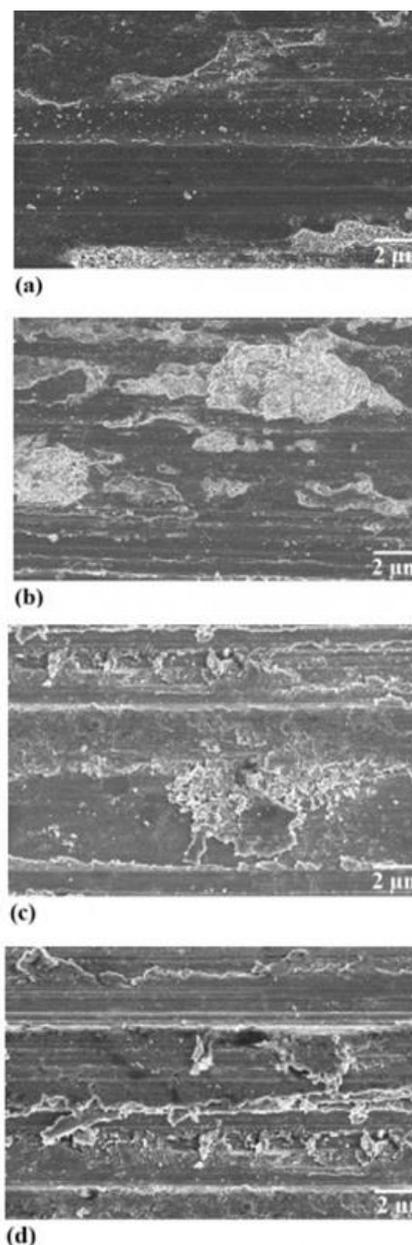
**Fig 3.** SEM examination of the worn-out surfaces at: (a)  $L = 10\text{ N}$ ,  $V = 2\text{ m/s}$ ,  $D = 1000\text{ m}$ ,  $R = 4\text{ wt-%}$  (b)  $L = 20\text{ N}$ ,  $V = 4\text{ m/s}$ ,  $D = 1500\text{ m}$ ,  $R = 4\text{ wt-%}$  (c)  $L = 30\text{ N}$ ,  $V = 3\text{ m/s}$ ,  $D = 500\text{ m}$ ,  $R = 4\text{ wt-%}$  (d)  $L = 40\text{ N}$ ,  $V = 1\text{ m/s}$ ,  $D = 2000\text{ m}$ ,  $R = 4\text{ wt-%}$
