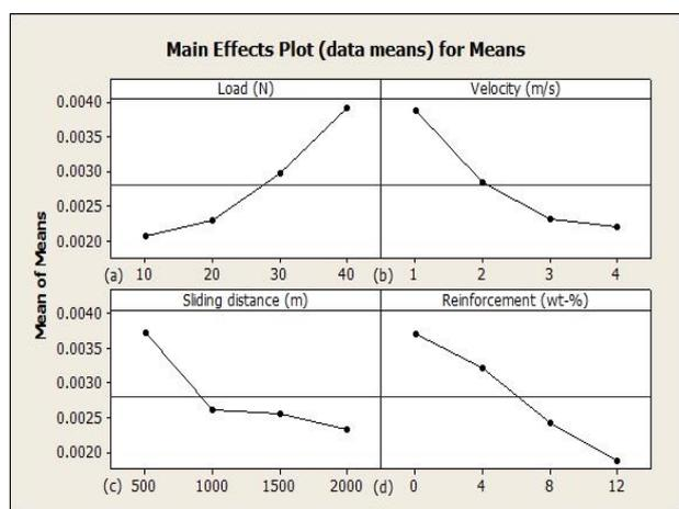
Fig 1. Main effect plots for means–Wear rate.
