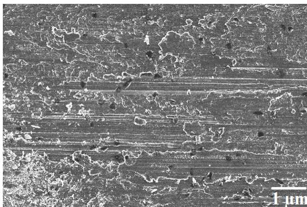
**Fig 4.** SEM examination of the worn-out surface at optimum condition.
