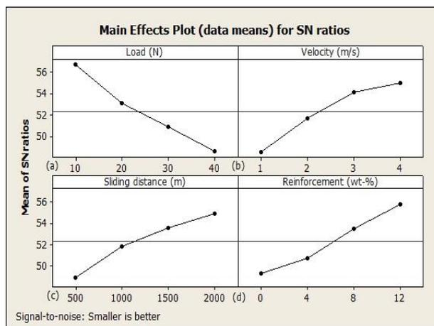
Fig 2. Main effect plots for S/N ratio–Wear rate.
