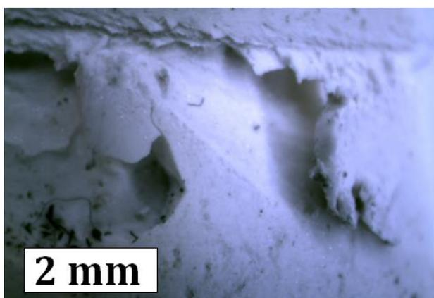
**Fig. 15.** Wear of the surface of MOM vulcanizate after tribological test under the load of 30 N.
