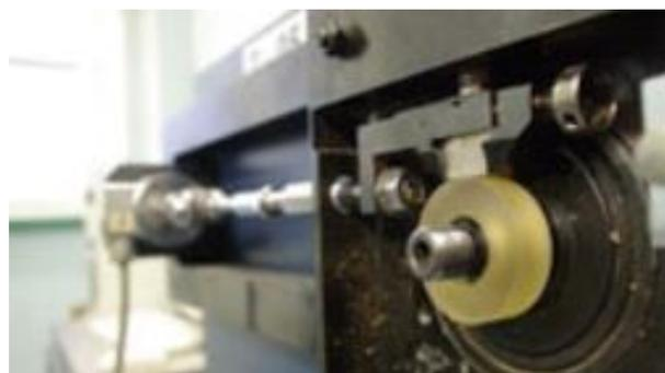
**Fig. 2.** Photograph of a T-05 tribo-tester.
