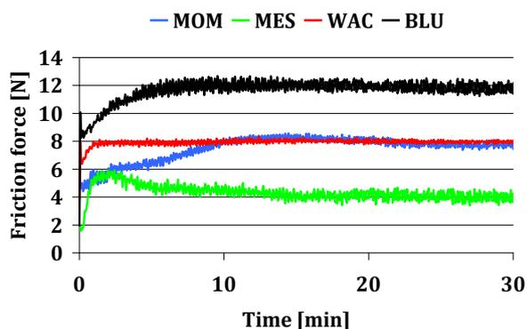
Fig. 3. Changes to the friction force in time for vulcanizates loaded with the force of 5 N.
