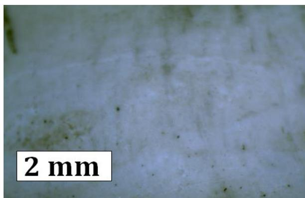
**Fig. 18.** The surface of MES vulcanizate after tribological test under the load of 30 N.
