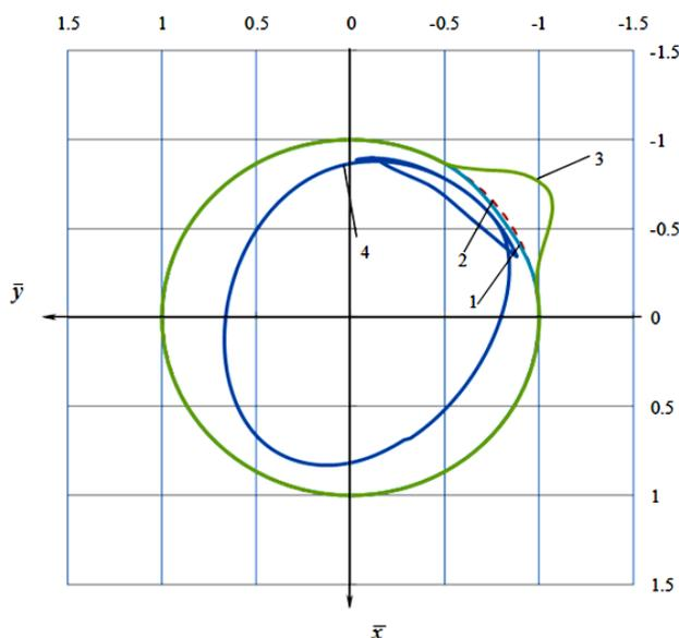
**Fig. 1.** Trajectory of the movement of the center of a rod journal in the bearing: 1 – theoretical wear diagram of the journal; 2 – unit circle; 3 – theoretical wear diagram of the bearing; 4 – trajectory of the journal.
