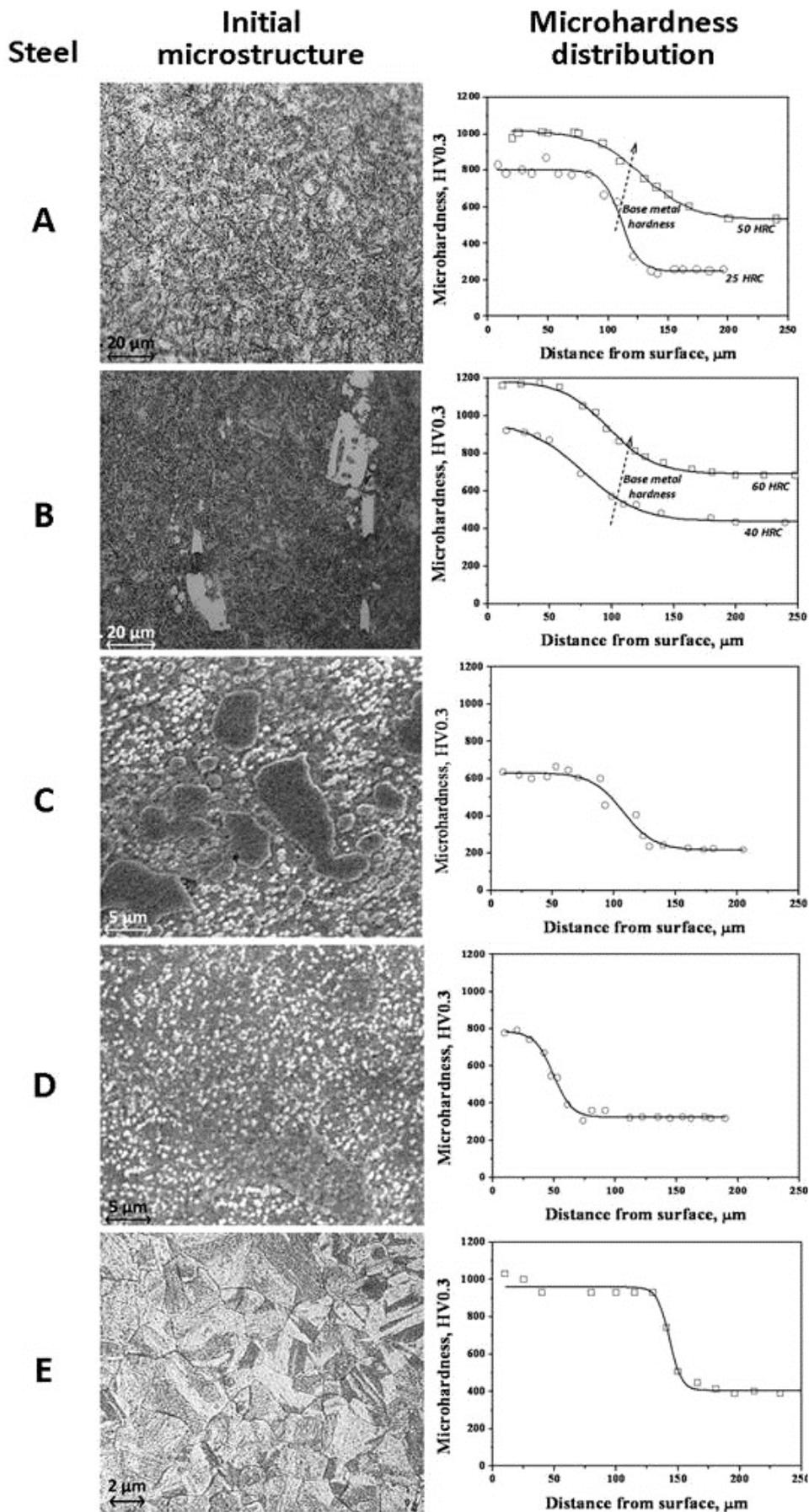
**Fig. 2.** Initial microstructure and in-depth microhardness distribution after nitrocarburising of the five (5) steel grades examined.
