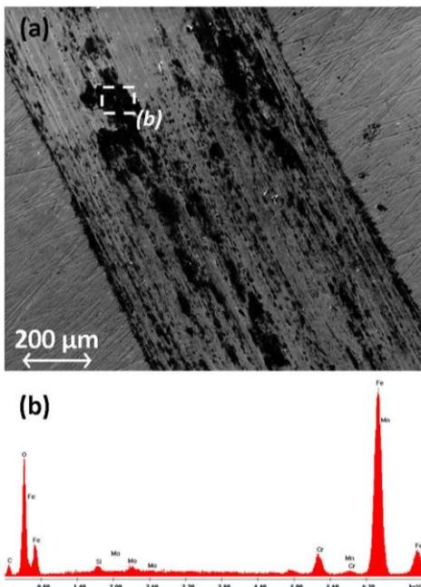
Fig. 5. (a) Characteristic SEM micrograph of the worn surface of heat-only-treated steel (A), tested in configuration (I) and (b) EDS spectrum of the area marked in (a).
