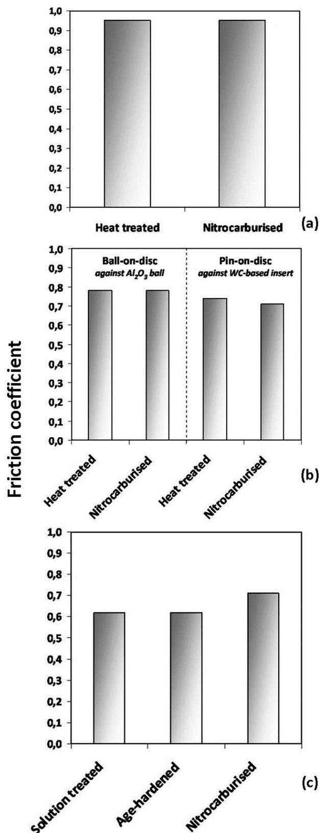
Fig. 3. Friction coefficient values for various tribosystems: (a) Steel (A) against Al<sub>2</sub>O<sub>3</sub> ball, (b) Steel (B) against Al<sub>2</sub>O<sub>3</sub> ball and against WC-based insert and (c) Steel (E) against WC-based insert.
