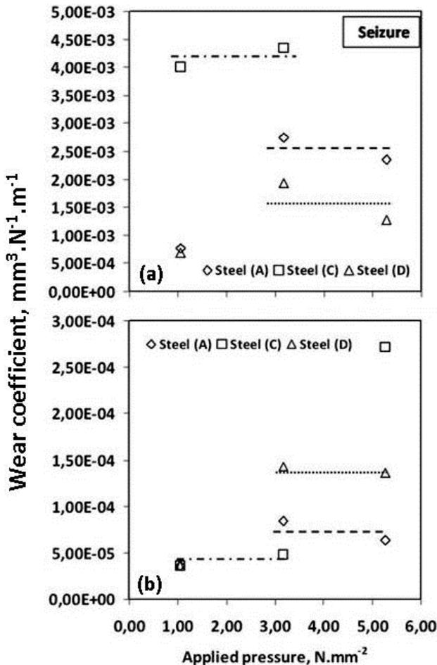
Fig. 7. Evolution of wear coefficient of the three steel grades examined in conformal configuration (III) versus the applied pressure: (a) In soft-annealing state, (b) after nitrocarburising.
