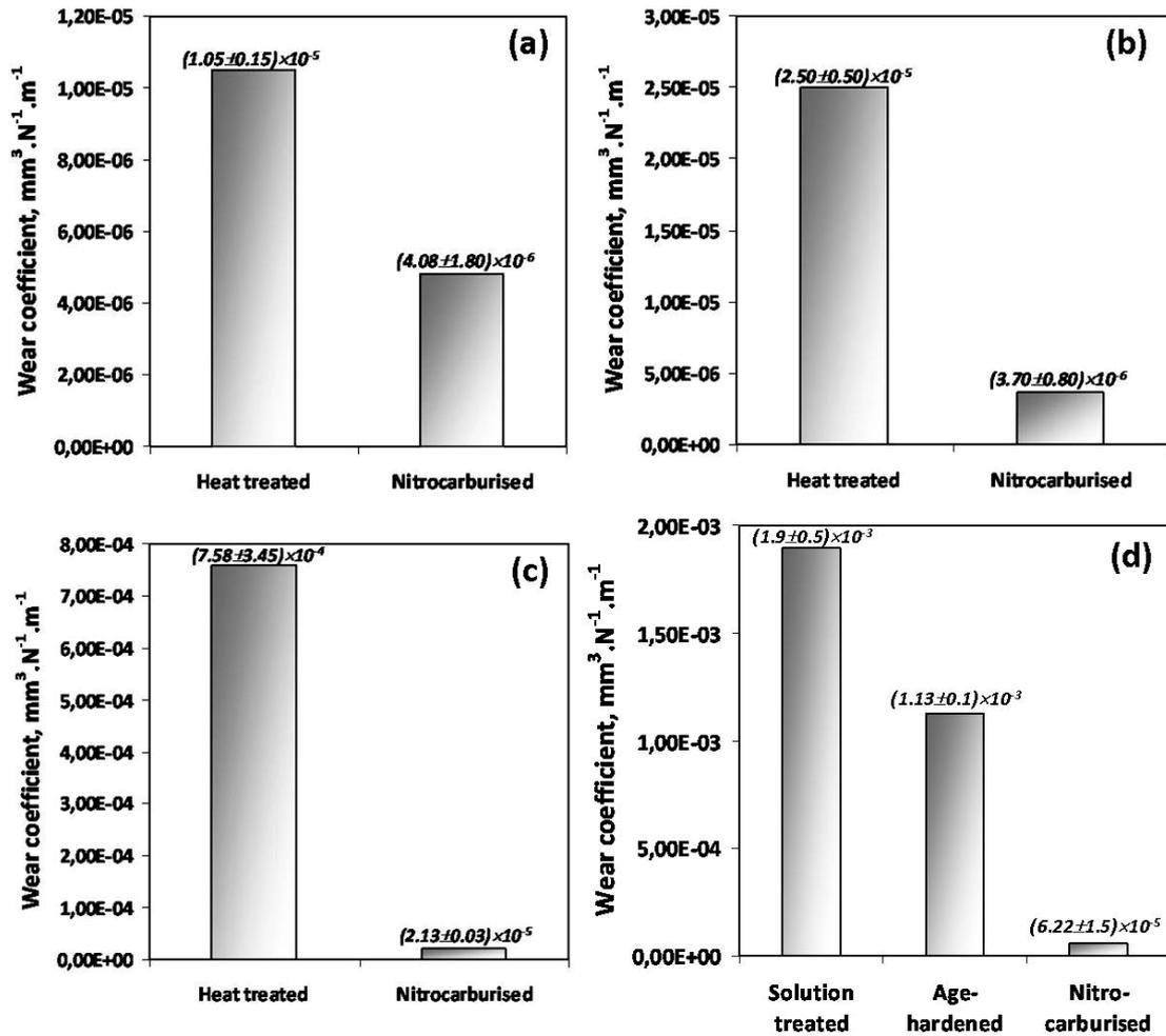
Fig. 4. Wear coefficient values for various tribosystems: (a) Steel (A) against Al<sub>2</sub>O<sub>3</sub> ball, (b) Steel (B) against Al<sub>2</sub>O<sub>3</sub> ball, (c) Steel (B) against WC-based insert and (d) Steel (E) against WC-based insert.
