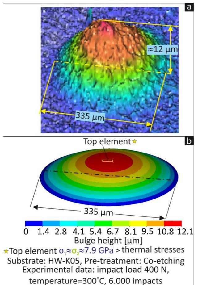
**Fig. 9.** (a) film bulge geometry after inclined impact test on NCD film on a substrate treated by Co-etching and (b) FEM calculated residual stresses for achieving the same bulge geometry.
