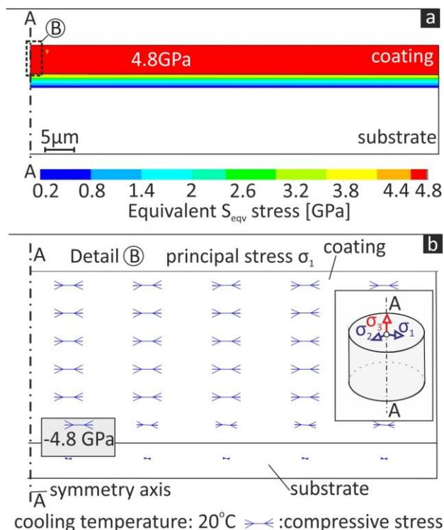
Fig. 5. (a) the developed equivalent stress field after cooling from the deposition temperature to the ambient one and (b) the relevant principal stress  $\sigma_1$  field.
