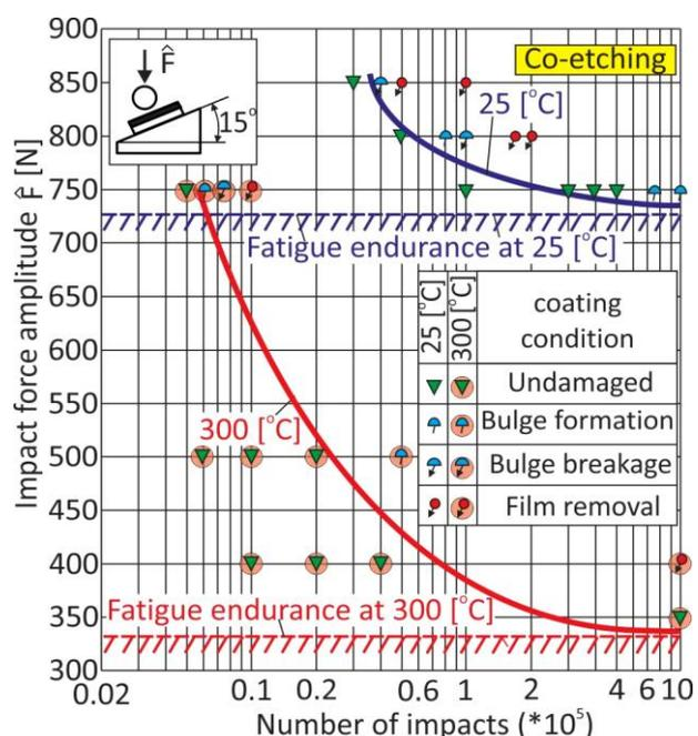
**Fig. 4.** NCD coating conditions after inclined impact tests with Co-etching substrate treatment.
