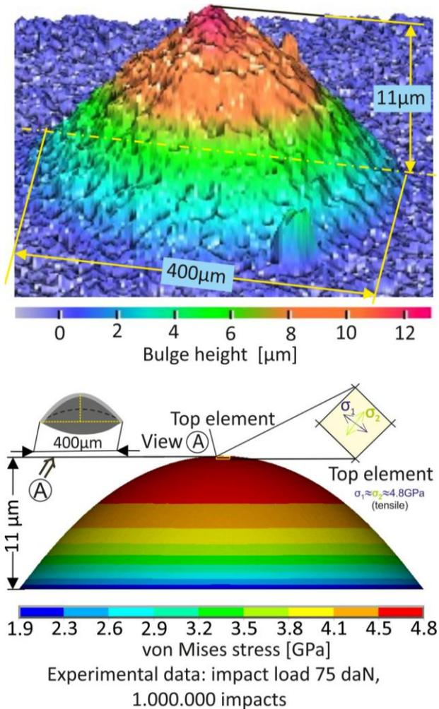
**Fig. 8.** Distribution of the measured displacement  $z$  and von Mises film stresses in the detached film region.
