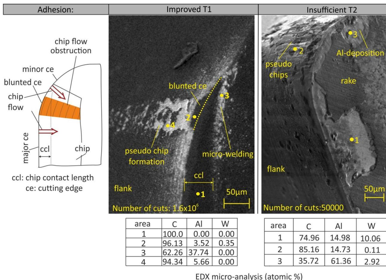
**Fig. 12.** SEM micro-graphs of NCD coated tools with improved adhesion (T1) after 1.6 million cuts and with insufficient adhesion (T2) after 50 thousand cuts.
