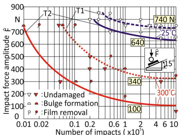
**Fig. 11.** Impact test results at various loads and temperatures for different film adhesion qualities.
