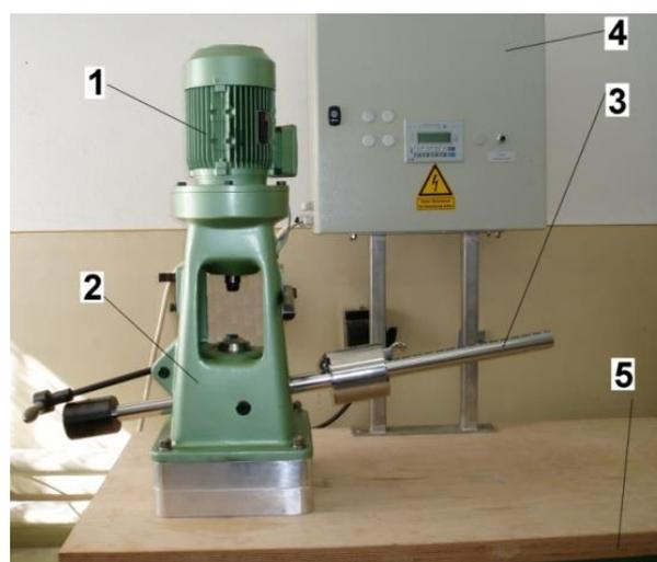
**Fig. 1.** The four ball machine.
