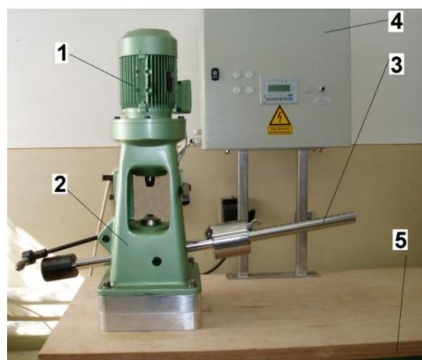
**Fig. 1.** The four ball machine.
