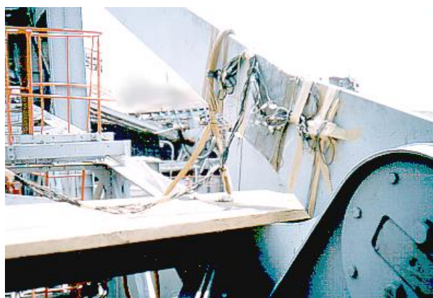
Fig. 6. Aspect of the measuring installation on one of the clamp dogs.
