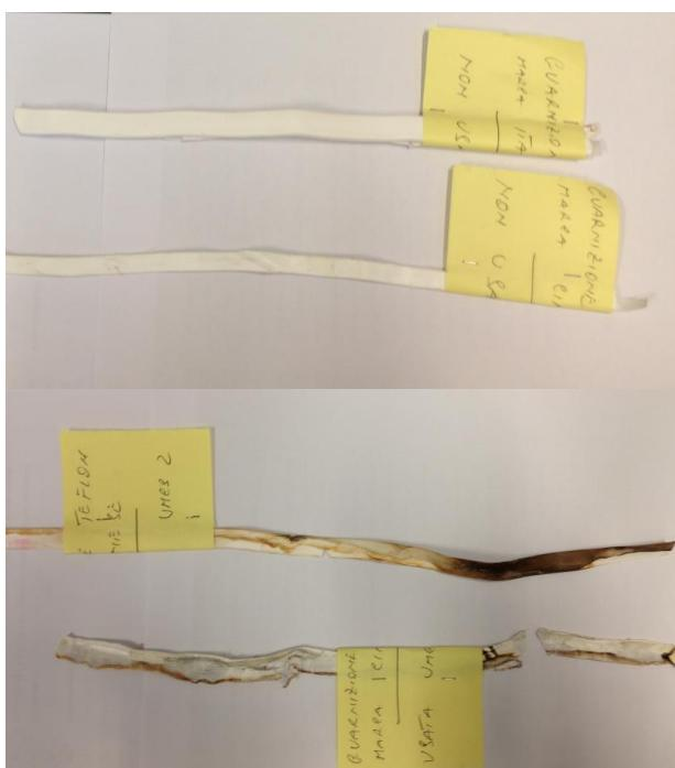
**Fig. 4.** PTFE tapes from both producers before (top) and after (down) their utilization inside the Ultrasonic Mold Cleaning Systems.
