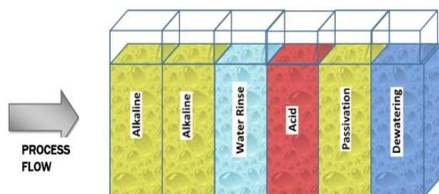
**Fig. 5.** Process stages and relative chemical baths in the Ultrasonic Mold Cleaning System [17].
