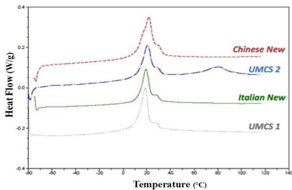
**Fig. 14.** Differential scanning calorimetry curves of *Italian New*, *Chinese New*, *UMCS 1* and *UMCS 2*.
