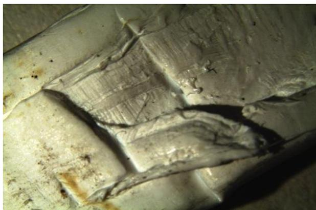
**Fig. 7.** An image by optical microscopy showing evidences of geometrical faults and partially altered surfaces in *Chinese New* sample (not existing in *Italian New* ones).
