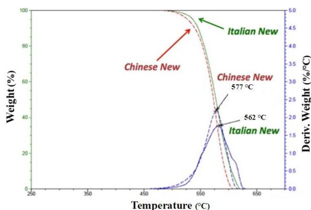
Fig. 12. Thermograms of *Italian New* (green line) and *Chinese New* (red line) samples.
