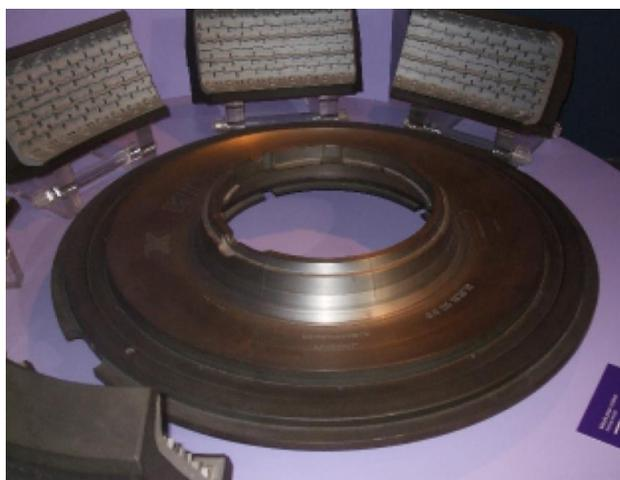
**Fig. 1.** Metal mold used in tires production and sections of tires (Courtesy Michelin).
