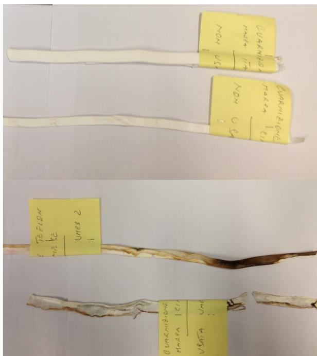
**Fig. 4.** PTFE tapes from both producers before (*top*) and after (*down*) their utilization inside the Ultrasonic Mold Cleaning Systems.
