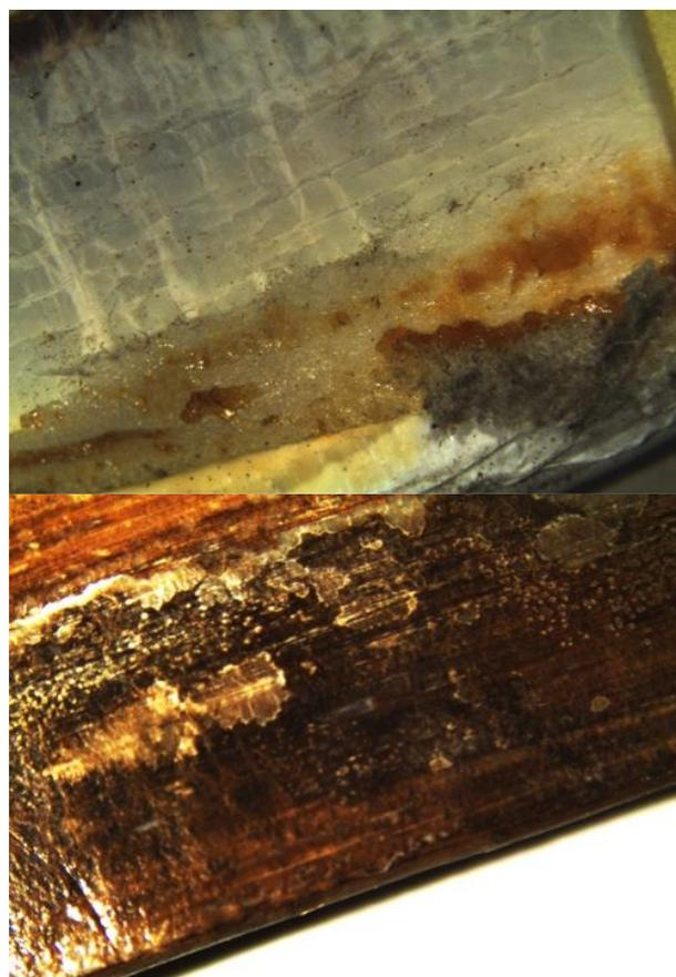
**Fig. 9.** Images by optical microscopy showing evidences of geometrical faults and partially altered surfaces in *UMCS1* (up) and *UMCS2* (down).
