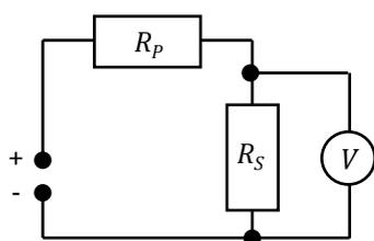
**Fig. 7.** Primarily designed electrical scheme:  $R_p$  - added resistance.
