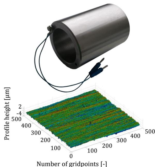
Fig. 2. Experimental piston with an example of its surface pattern.
