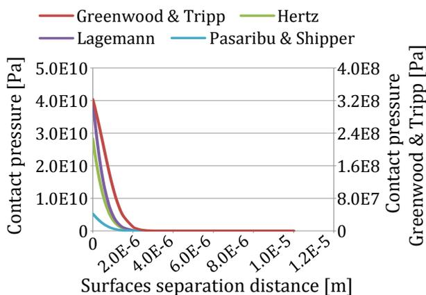
**Fig. 4.** Contact pressure dependence on surfaces separation.
