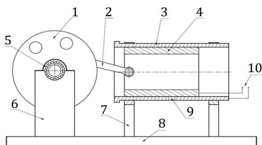
**Fig. 8.** Test rig scheme: 1 - crankshaft powered by electric engine, 2 - connecting rod, 3 - piston liner, 4 - experimental engine, 5 - crankshaft mount, 6 - crankshaft bearing housing, 7 - piston liner support, 8 - base, 9 - oil intake, 10 - cables for electric circuit connection.
