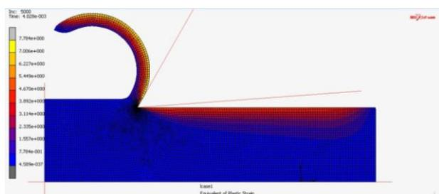
Fig. 3. Chip morphology and plastic strain.
