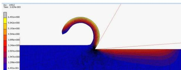
**Fig. 7.** Chip morphology and plastic strain in the simulation with Johnson-Cook material model.
