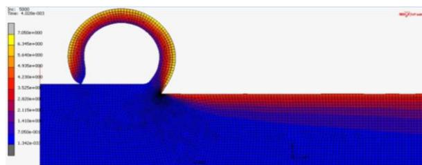
Fig. 1. Plastic strain in workpiece and chip.
