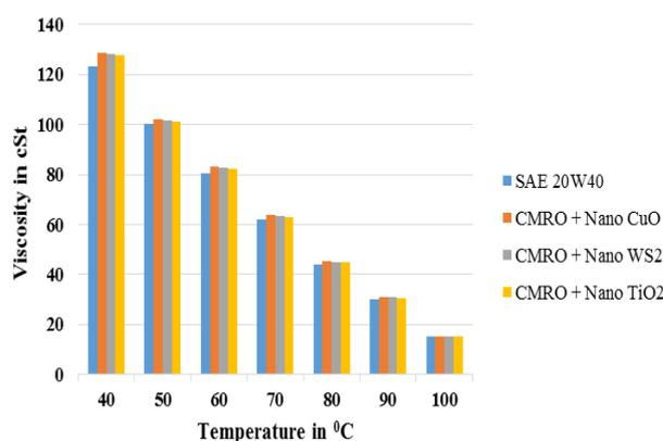
**Fig. 7** Viscosity (cSt) of Lubricating oils.
