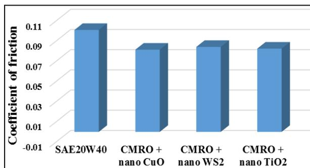
Fig. 4. Coefficient of friction for various lubricating oils.
