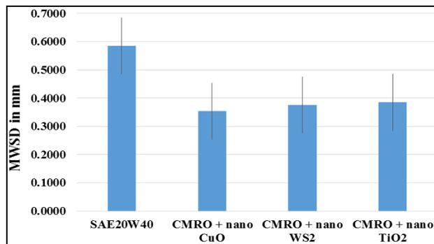
**Fig. 5.** Mean wear scar diameter of lubricating oils.
