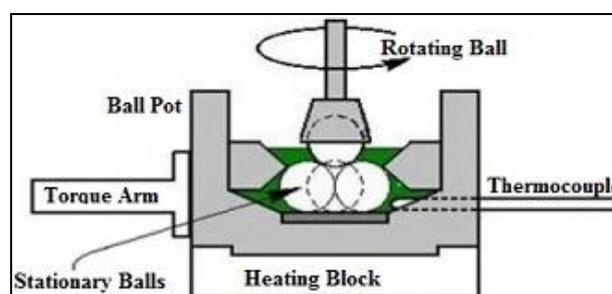
**Fig. 2.** Schematic diagram of Four ball tribometer.
