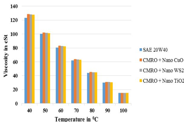
**Fig. 7** Viscosity (cSt) of Lubricating oils.
