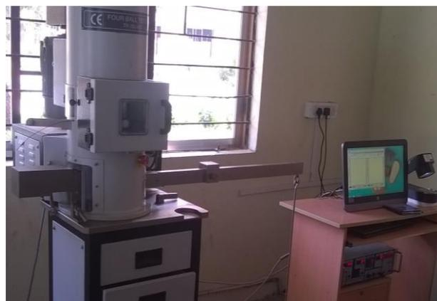
**Fig. 1.** Four ball tribometer.
