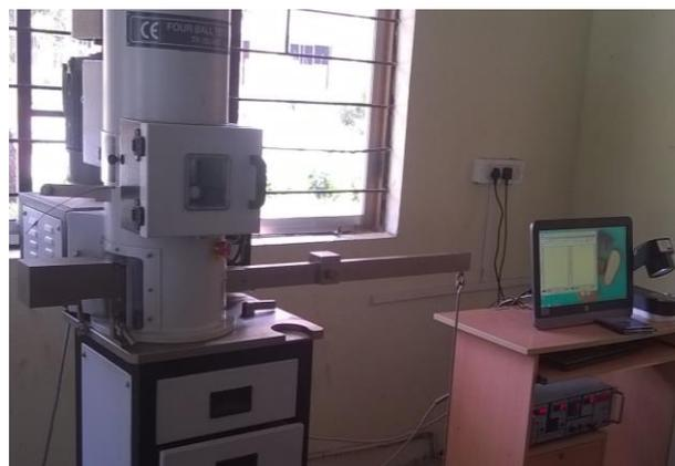
**Fig. 1.** Four ball tribometer.
