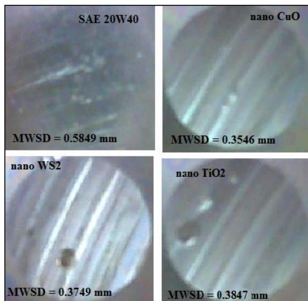
**Fig. 6.** Wear scar image of lubricating oils (Magnification 50X).
