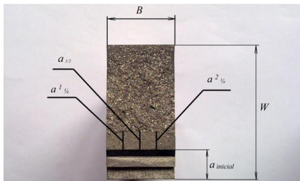
Fig. 13. One specimen after breaking
