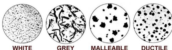
Fig. 1. Example of microstructures.
