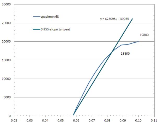
**Fig. 10.** Procedure for obtaining  $P_Q$  (ASTM E1820)
