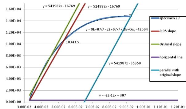
**Fig. 12.** Procedure for  $J$  calculation (ASTM E1820).
