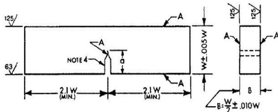
Fig. 6. Bend specimen with an EDM notch (ASTM 399).
