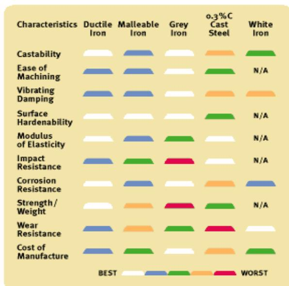
Fig. 2. Comparing different forms of cast iron.
