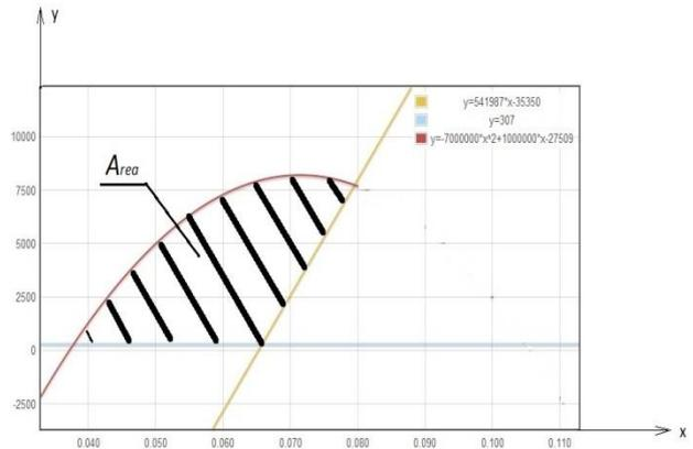
**Fig. 11.** Procedure for  $J$  calculation (ASTM E813)
