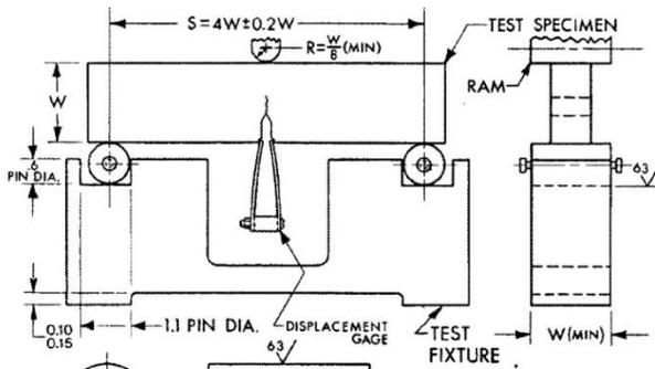
Fig. 7. Bend test fixture design (ASTM 399).
