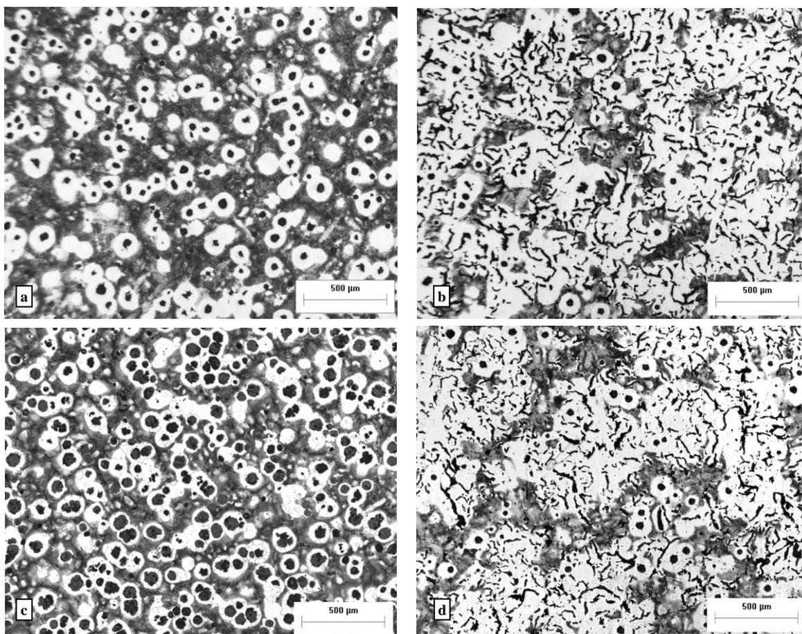
**Fig. 5.** OM micrographs after Nital etching of: 1st batch SGI specimen (a); 1st batch CGI specimen (b); 2nd batch SGI specimen (c); 2nd batch CGI specimen (d). Graphite nodules and worms (black), ferrite islands (white) and perlite (grey) are evident.
