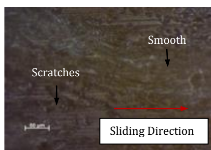
Fig. 21. Contact Surface of PRBF in Wet Test at 7.2 m/sec and 50 N.
