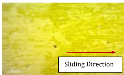
Fig. 16. Contact Surface of N66a in Dry Test at 7.2 m/sec and 50 N.
