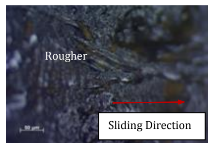
Fig. 20. Contact Surface of PRBF in Dry Test at 7.2 m/sec and 50 N.
