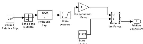
Fig. 11. Simulink model for single wheel drum brake.
