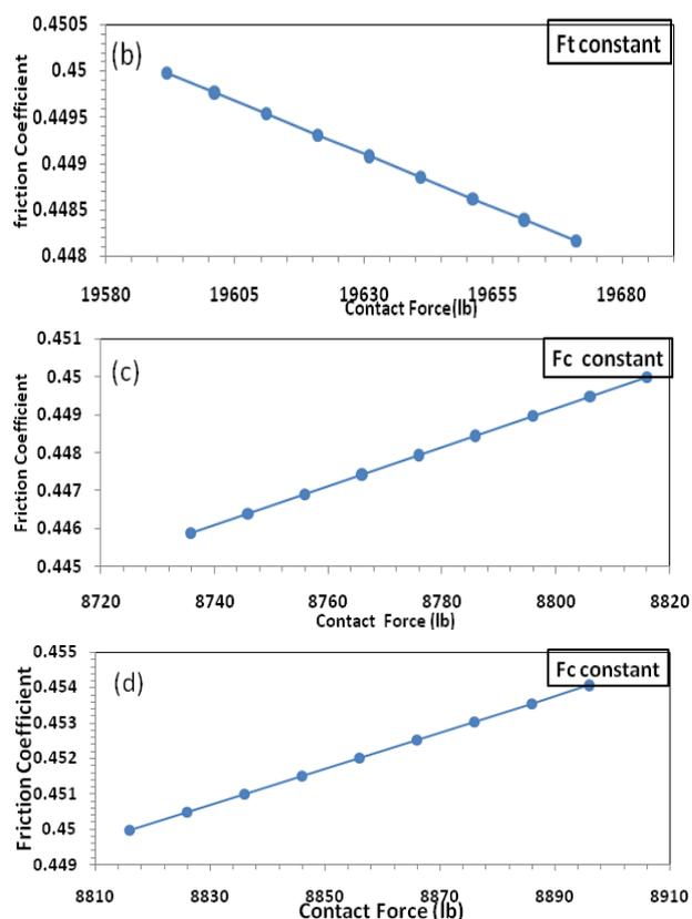
Fig. 16 (a-d). Friction Coefficient profiles for variations in contact force for disc brake.
