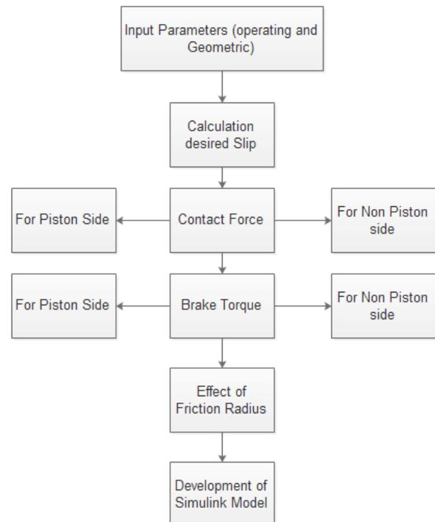
Fig. 10. Algorithm for friction coefficient estimation.
