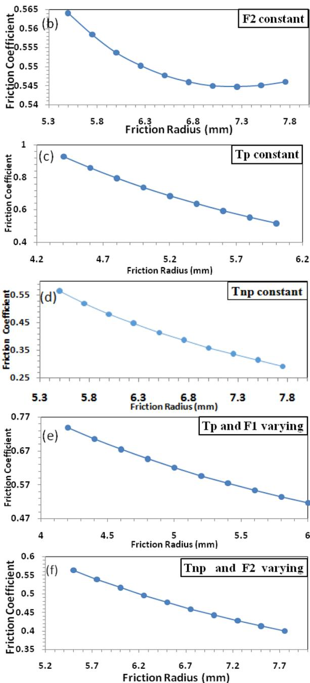
Fig 18 (a-f).Friction coefficient profiles for variations in friction radius for disc brake.
