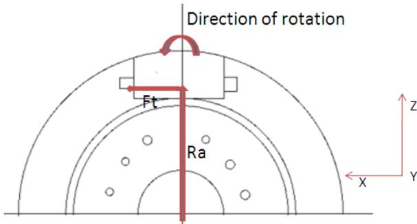
Fig. 6. Tangential force at the caliper.
