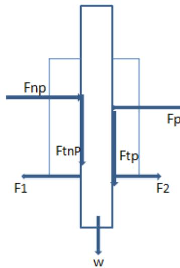
Fig. 4. Forces with variations in active friction radius.
