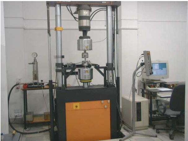
**Fig. 5.** Uniaxial loading tensile servo-hydraulic testing machine INSTRON® 1343.
