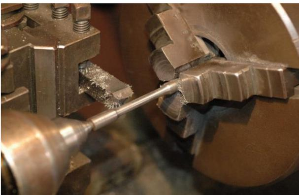
**Fig. 6.** “Dog bone” shape for a tensile specimen.
