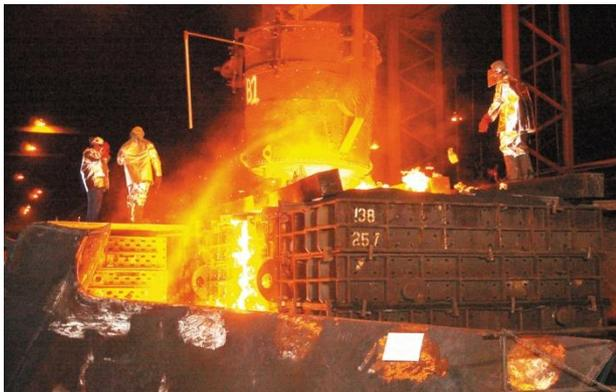
Fig. 2. Production of cast iron in factory (courtesy US Navy).
