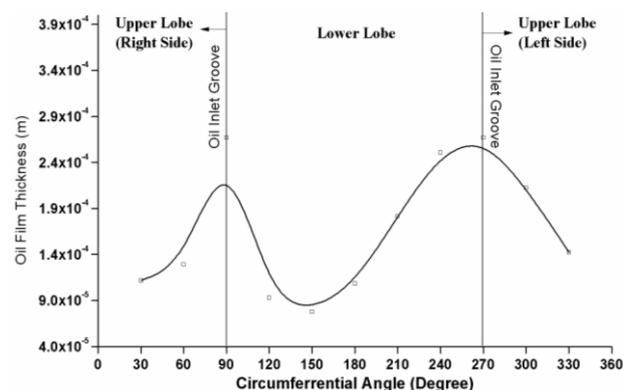
**Fig. 8.** Variation of oil film thickness plot for an elliptical journal bearing under study.
