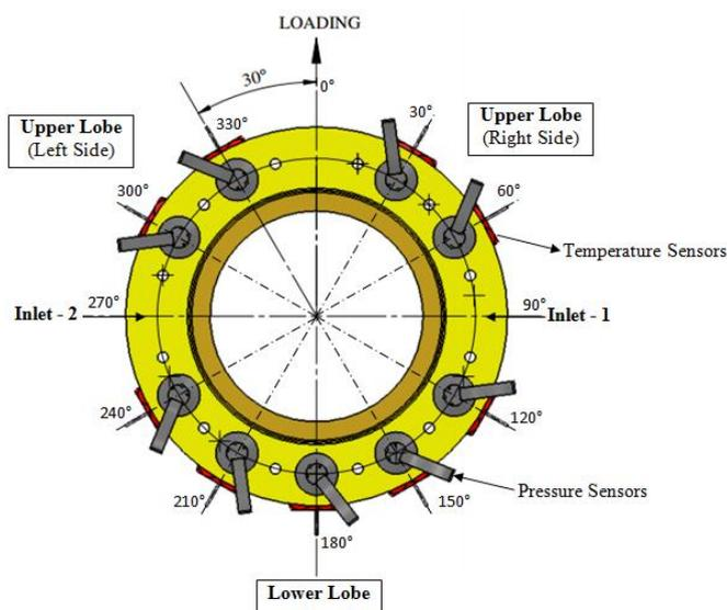
**Fig. 4.** Location and position of pressure and temperature sensor along the circumference of bearing.
