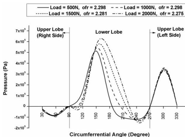
**Fig. 7.** Variation of pressure along the circumference of elliptical bearing at the central plane at 5000 rpm for different load = 500, 1000, 1500, 2000 N load for lubricating oil - 3.
