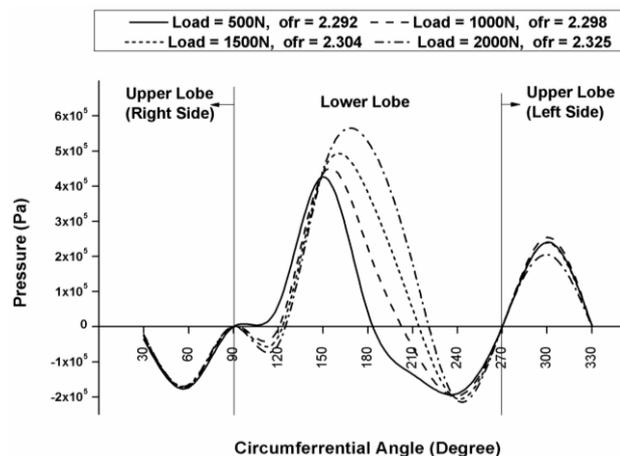
**Fig. 6:** Variation of pressure along the circumference of elliptical bearing at the central plane at 5000 rpm for different load = 500, 1000, 1500, 2000 N load for lubricating oil - 2.
