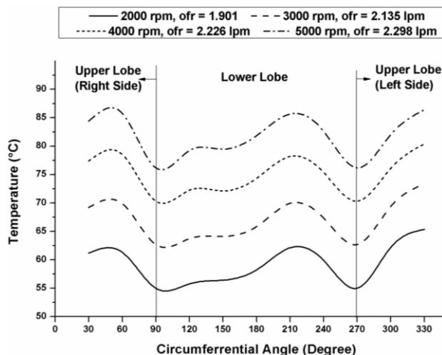
**Fig. 13:** Effect of variation of speed= 2000, 3000, 4000 and 5000 rpm on the oil film temperature at the central plane of elliptical bearing for oil - 2.
