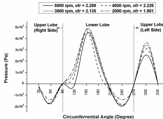
**Fig. 12.** Effect of variation of speed= 2000, 3000, 4000 and 5000 rpm on the lubricating oil pressure at the central plane of elliptical bearing for oil - 2 only.
