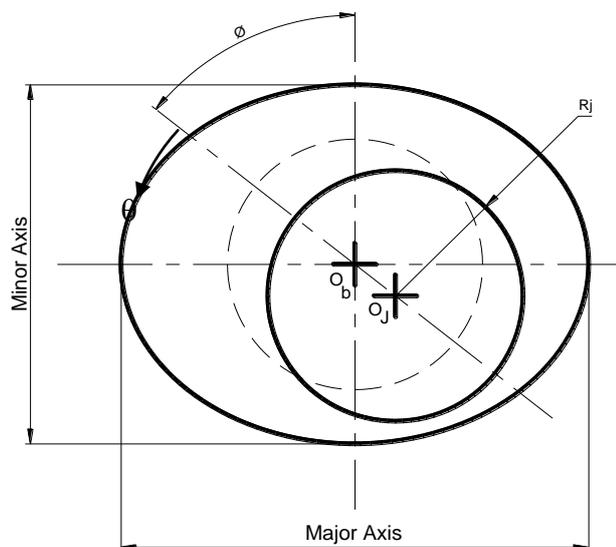
**Fig. 1.** Schematic diagram of elliptical profile journal bearing.
