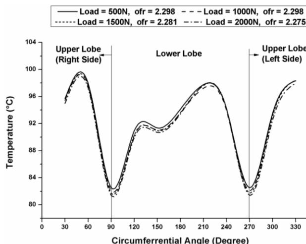
**Fig. 11:** Variation of temperature along the circumference of elliptical bearing at the central plane at 5000 rpm for different load = 500, 1000, 1500, 2000 N load for lubricating oil - 3.
