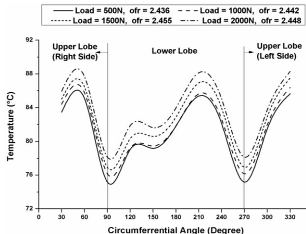
**Fig. 10.** Variation of temperature along the circumference of elliptical bearing at the central plane at 5000 rpm for different load = 500, 1000, 1500, 2000 N load for lubricating oil - 2.
