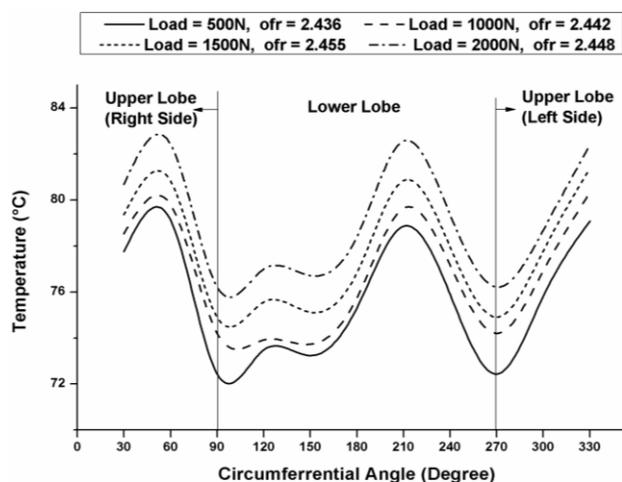
**Fig. 9.** Variation of temperature along the circumference of elliptical bearing at the central plane at 5000 rpm for different load = 500, 1000, 1500, 2000 N load for lubricating oil - 1.
