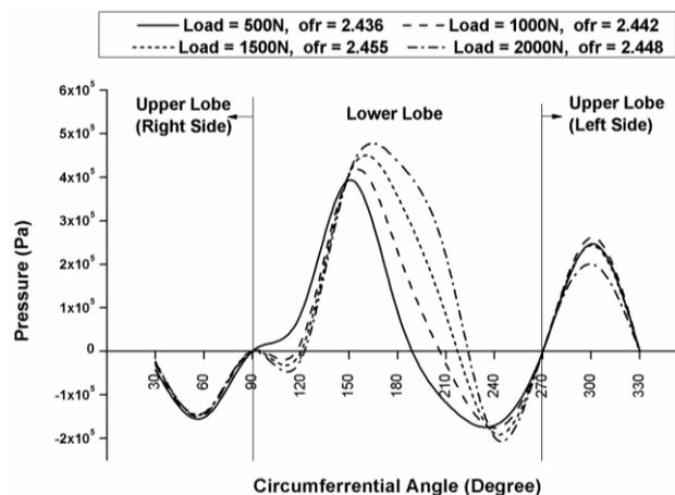
**Fig. 5.** Variation of pressure along the circumference of elliptical bearing at the central plane at 5000 rpm for different load = 500, 1000, 1500, 2000 N load for lubricating oil - 1.
