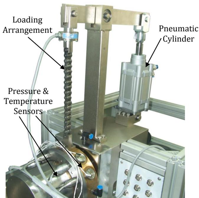
**Fig. 2.** Non-Circular journal bearing test rig for measurement of pressure and temperature at different load.
