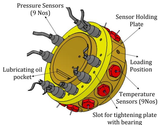
**Fig. 3.** The Elliptical test bearing equipped with pressure and temperature Sensor.
