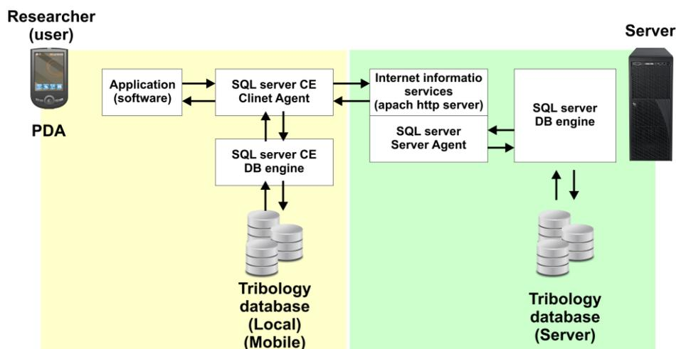
Fig. 11. Replication architecture.
