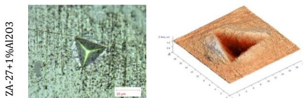
**Fig. 6.** Indentation imprints analysed by optical and AFM microscopy [10].
