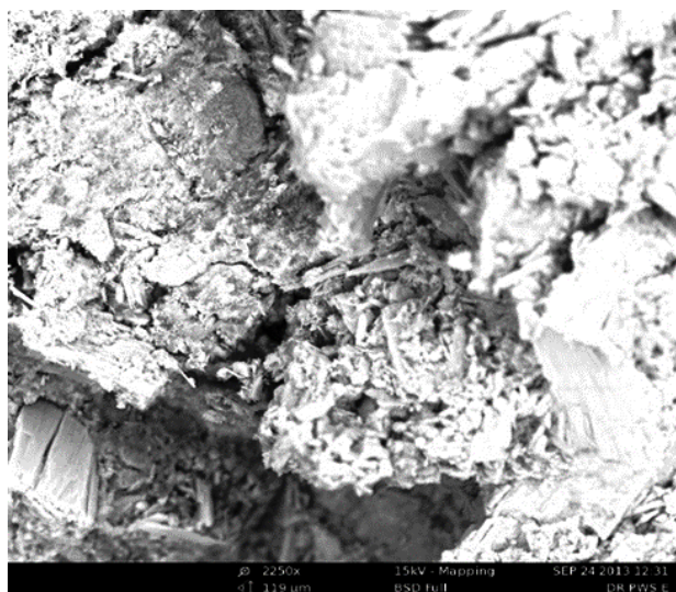
Fig. 7. SEM/EDS microstructure of PKS/resin composite with 87 wt.% particle.
